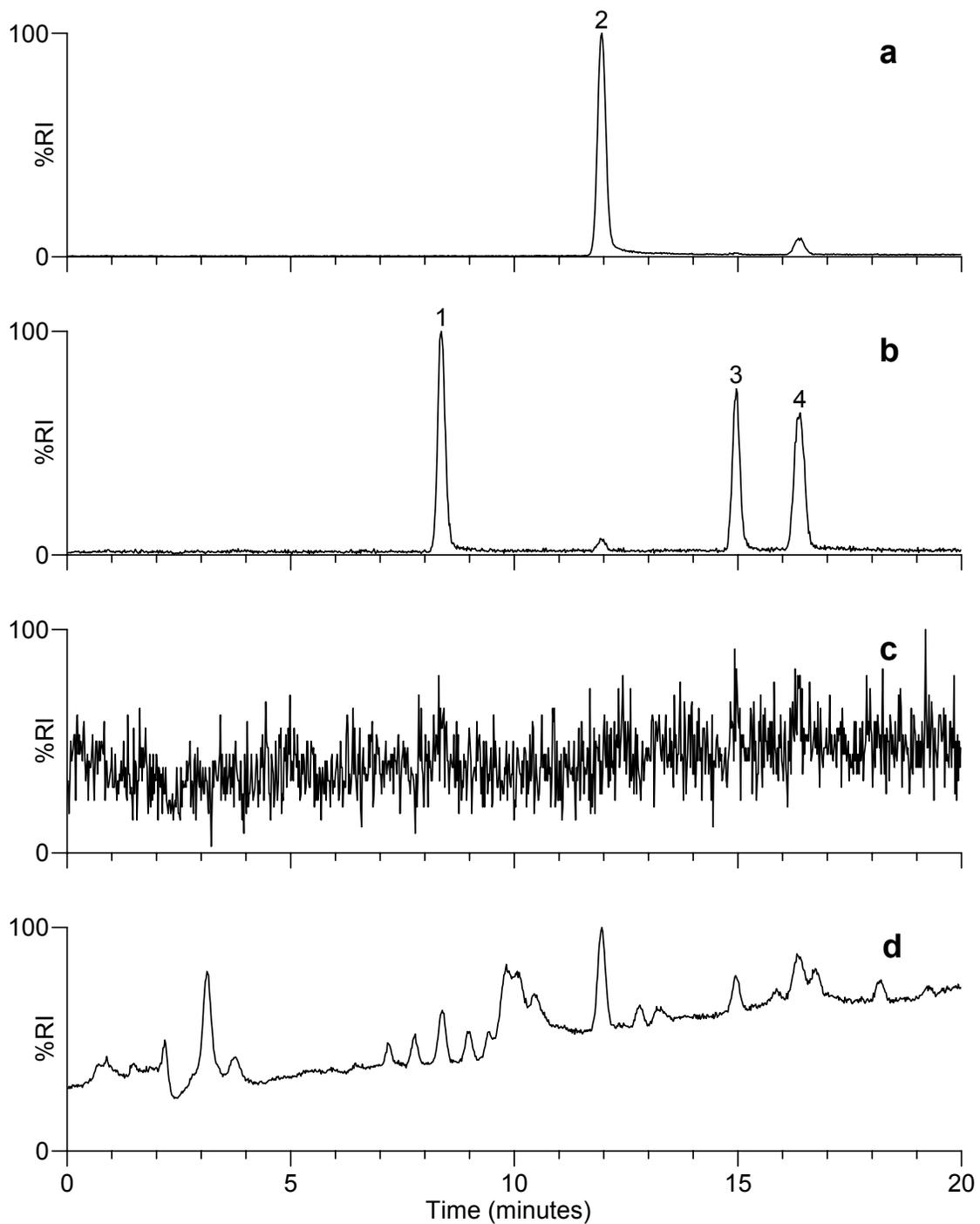
**Figure 3.** Reconstructed-ion-current chromatograms for a)  $m/z$  183, b)  $m/z$  99, c)  $m/z$  97 and d) total-ion-current chromatogram obtained during LC-ESI-MS analysis of an extract of a Dacron swab sample spiked at the  $20 \mu\text{g/g}$  level with GB (1), TEP (2), GF (3) and GD (4).
