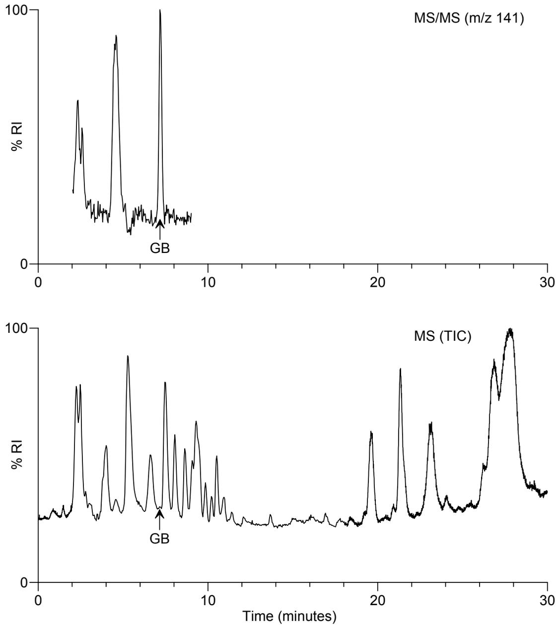
**Figure 8.** LC-ESI-MS total-ion-current chromatogram (lower) and LC-ESI-MS/MS chromatogram for the product ions of  $m/z$  141 (upper) obtained during analysis of an extract of a office carpet sample spiked at the  $4 \mu\text{g/g}$  level with GB, TEP, GF and GD.
