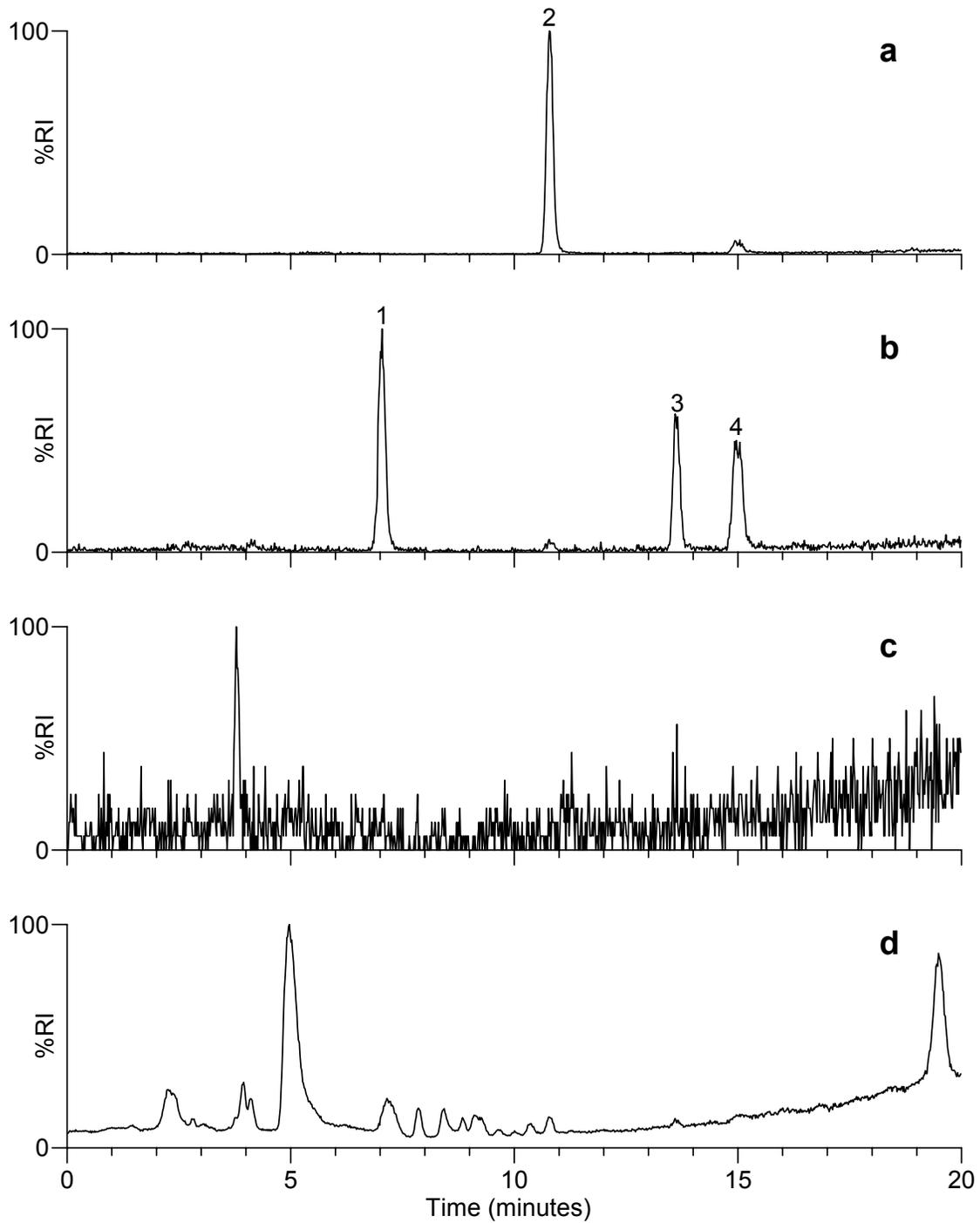
**Figure 1.** Reconstructed-ion-current chromatograms for a)  $m/z$  183, b)  $m/z$  99, c)  $m/z$  97 and d) total-ion-current chromatogram obtained during LC-ESI-MS analysis of an extract of an office carpet sample spiked at the  $4 \mu\text{g/g}$  level with GB (1), TEP (2), GF (3) and GD (4).
