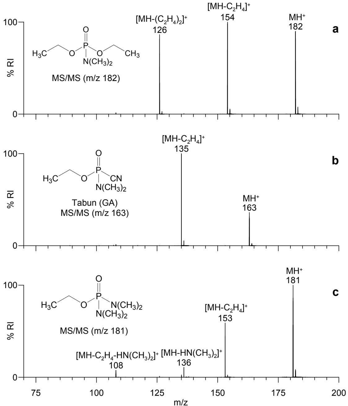
**Figure 11.** Product ion mass spectra obtained for a) diethyl dimethylphosphoramidate (m/z 182, Collision energy: 10V), b) GA (m/z 163, Collision energy: 7V) and c) ethyl tetramethylphosphoramidate (m/z 181, Collision energy: 10V) during LC-ESI-MS/MS analysis of an office carpet sample spiked with munitions grade GA (0.5 to 5  $\mu\text{g/g}$  per component).
