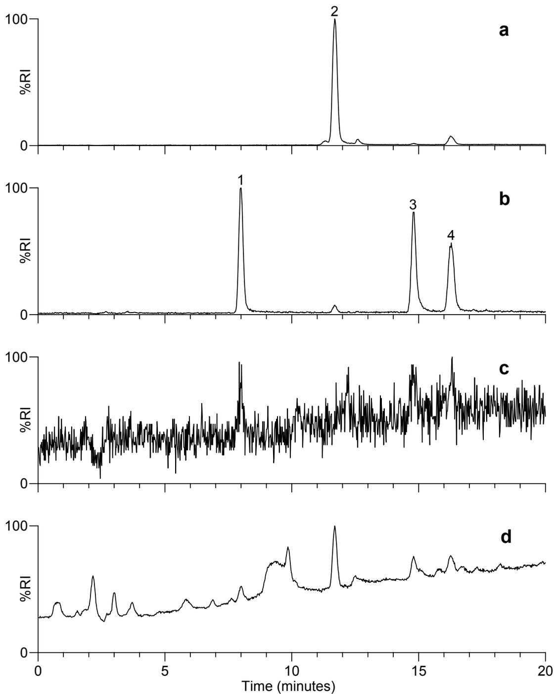
**Figure 6.** Reconstructed-ion-current chromatograms for a)  $m/z$  183, b)  $m/z$  99, c)  $m/z$  97 and d) total-ion-current chromatogram obtained during LC-ESI-MS analysis of an extract of an office fabric (100% nylon) sample spiked at the  $13 \mu\text{g/g}$  level with GB (1), TEP (2), GF (3) and GD (4).
