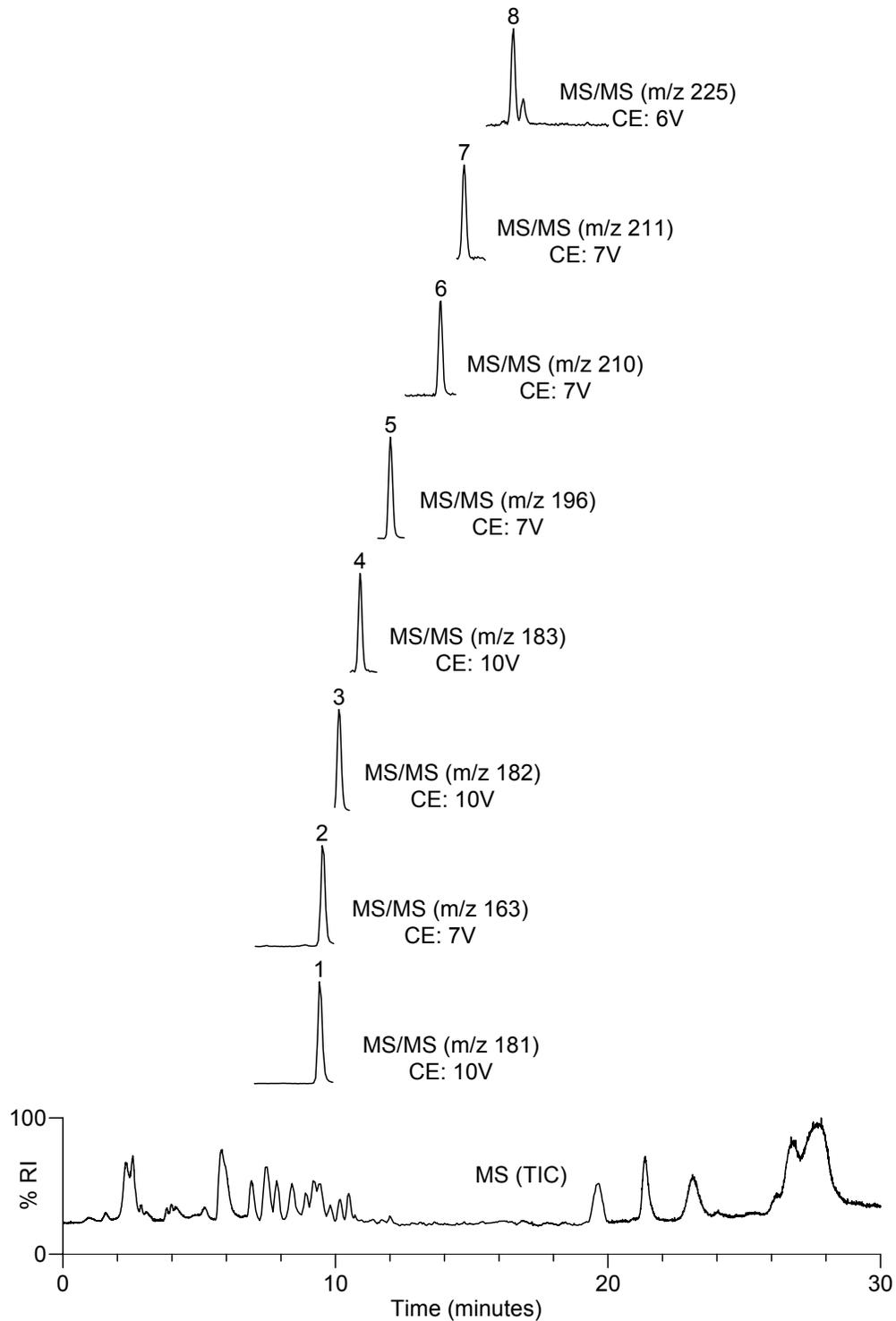
**Figure 10.** LC-ESI-MS (lowest) and LC-ESI-MS/MS chromatograms (above) of an extract of an office carpet spiked with munitions grade GA (0.5 – 5 µg/g per component). Components 1 to 8 identified in Table 2. (CE: Collision energy).
