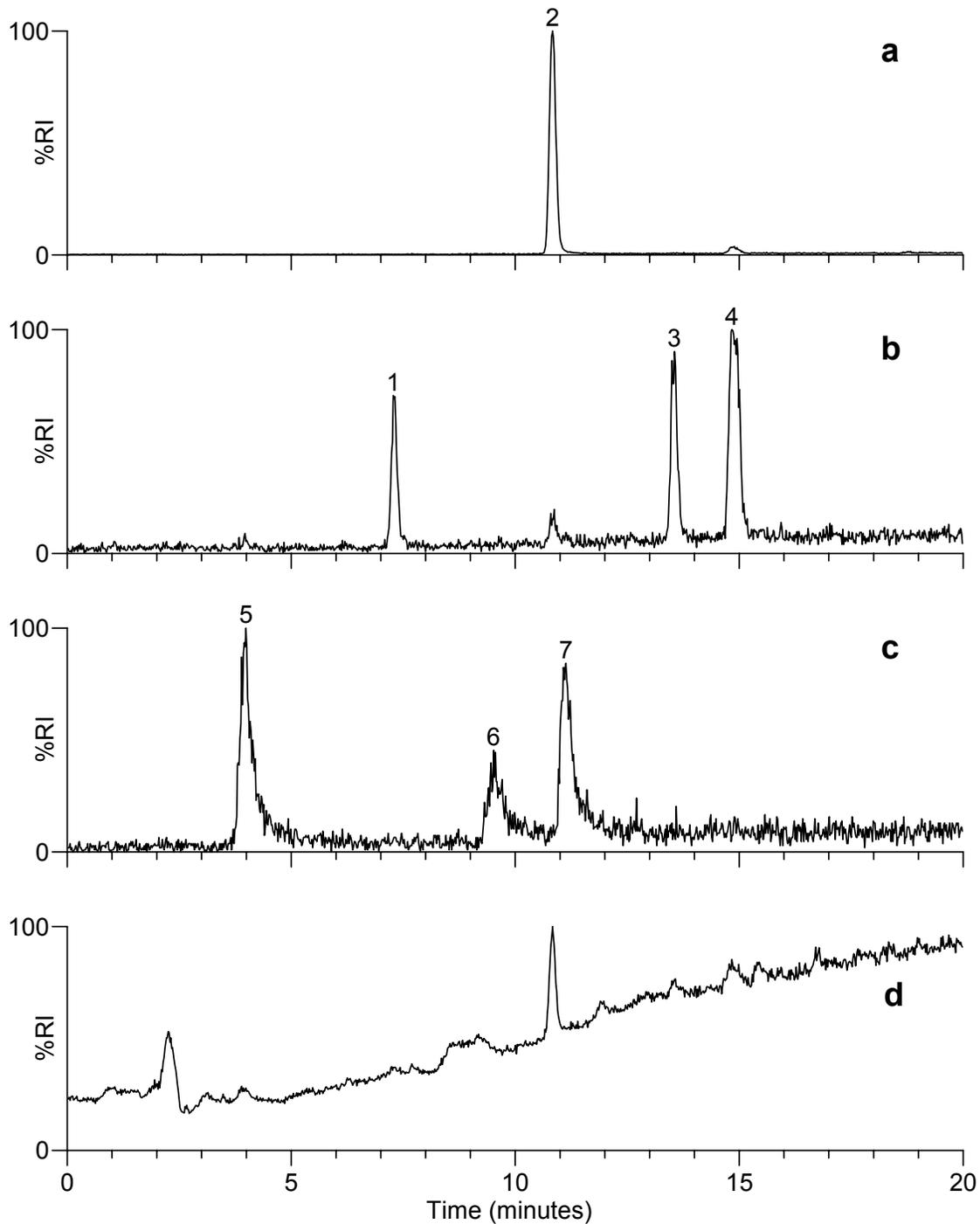
**Figure 2.** Reconstructed-ion-current chromatograms for a)  $m/z$  183, b)  $m/z$  99, c)  $m/z$  97 and d) total-ion-current chromatogram obtained during LC-ESI-MS analysis of an extract of a photocopier paper sample spiked at the  $8 \mu\text{g/g}$  level with GB (1), TEP (2), GF (3) and GD (4). Isopropyl methylphosphonic acid (5), cyclohexyl methylphosphonic acid (6) and pinacolyl methylphosphonic acid (7), the hydrolysis products of GB, GF and GD, respectively, were also observed.
