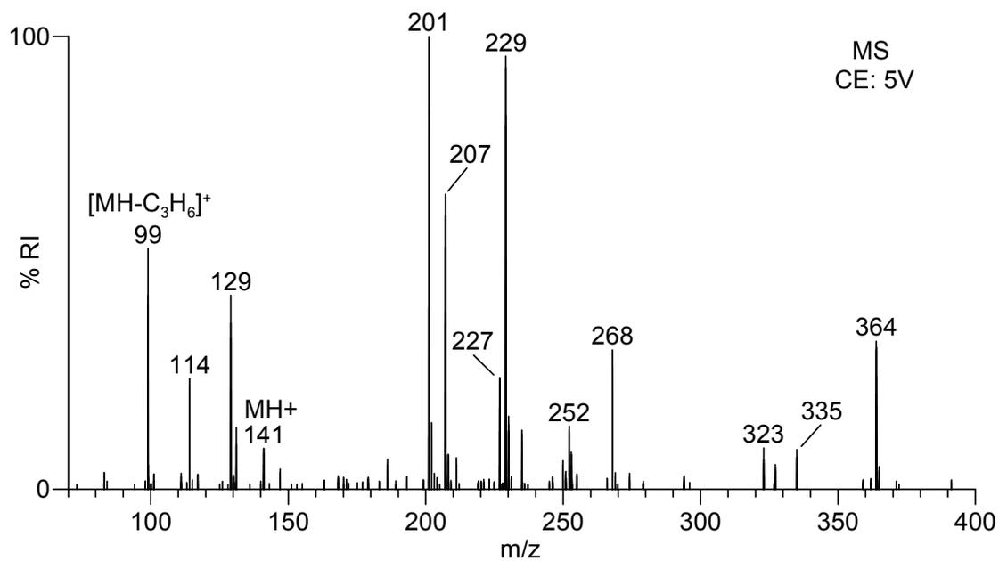
**Figure 9.** ESI-MS (lower) and ESI-MS/MS (upper) data obtained at the retention time for GB. Data were obtained during analysis of an extract of an office carpet sample spiked at the 4  $\mu\text{g/g}$  level with GB, TEP, GF and GD. (CE: Collision energy).
