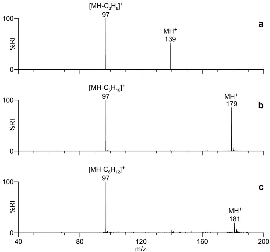
**Figure 7.** Product ion mass spectra obtained for protonated molecular ions of a) isopropyl methylphosphonic acid (m/z 139), b) cyclohexyl methylphosphonic acid (m/z 179) and c) pinacolyl methylphosphonic acid (m/z 181) during LC-ESI-MS/MS analysis of an extract of a photocopy paper sample spiked at the 8  $\mu\text{g/g}$  level with GB, TEP, GF and GD. (Collision energy: 4V).
