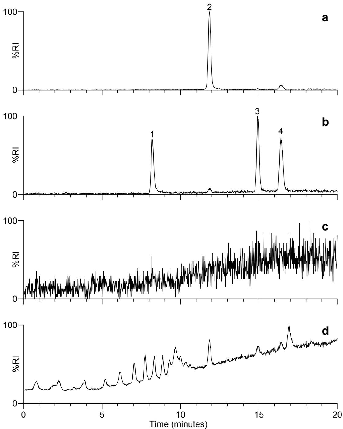
**Figure 5.** Reconstructed-ion-current chromatograms for a)  $m/z$  183, b)  $m/z$  99, c)  $m/z$  97 and d) total-ion-current chromatogram obtained during LC-ESI-MS analysis of an extract of an office fabric (56% nylon/44% polyester) sample spiked at the  $9 \mu\text{g/g}$  level with GB (1), TEP (2), GF (3) and GD (4).
