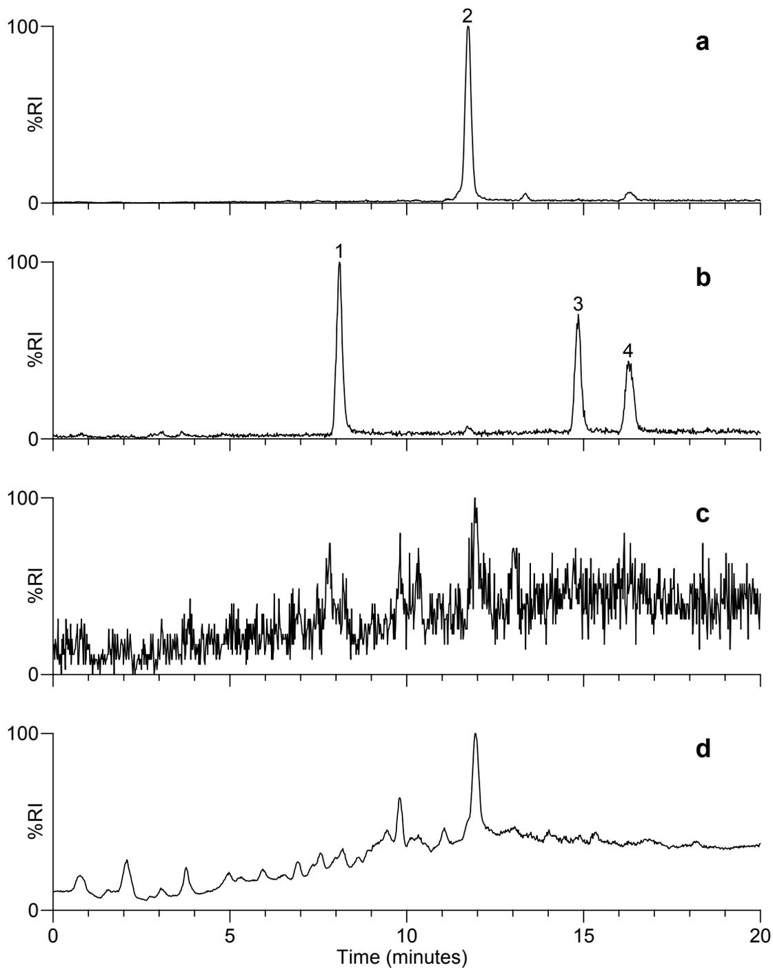
**Figure 4.** Reconstructed-ion-current chromatograms for a)  $m/z$  183, b)  $m/z$  99, c)  $m/z$  97 and d) total-ion-current chromatogram obtained during LC-ESI-MS analysis of an extract of a latex painted drywall sample spiked at the  $12 \mu\text{g/g}$  level with GB (1), TEP (2), GF (3) and GD (4).
