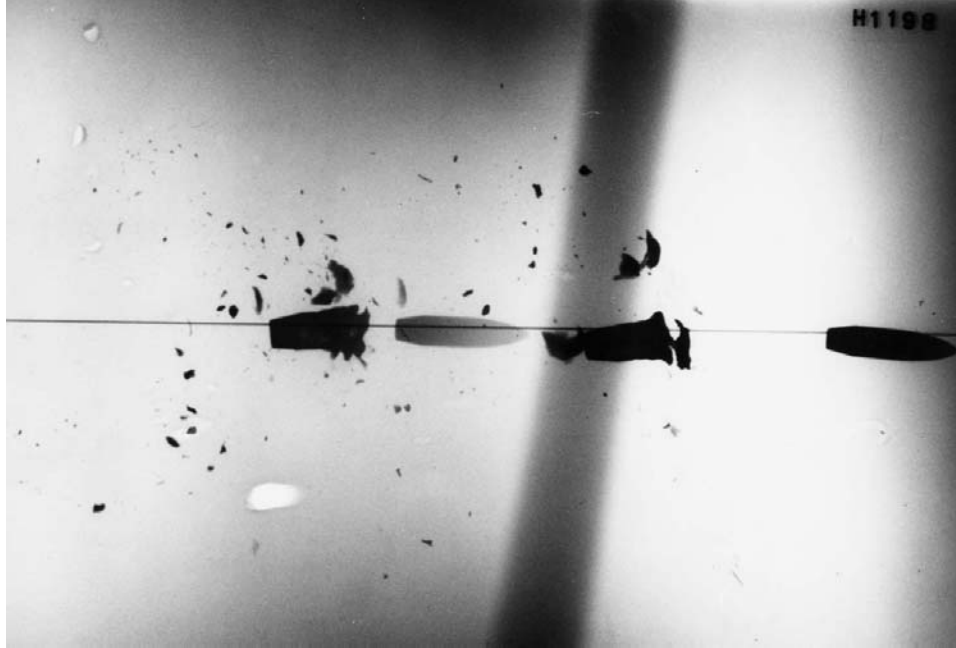
Figure 4. Horizontal x-ray view 0.5 APM2 ammunition
