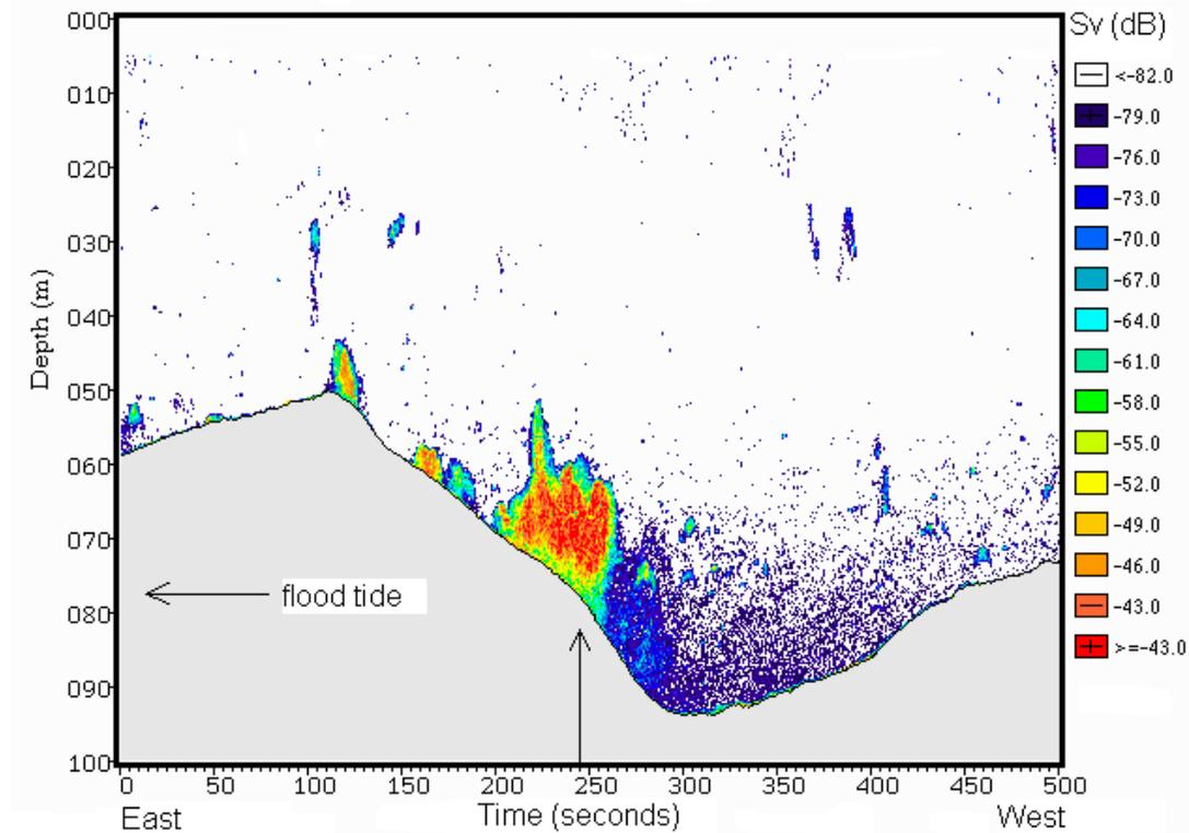
**Figure 1** 200 kHz volume back-scatter vs. depth and time echogram showing near-seabed fish schools in western Knight Inlet. Echogram starts 0908 PST, 19 Nov., 2002, with ship westbound during flood (eastbound) tide. Vertical arrow denotes time of multibeam sonar snapshot shown in Fig. 2.
