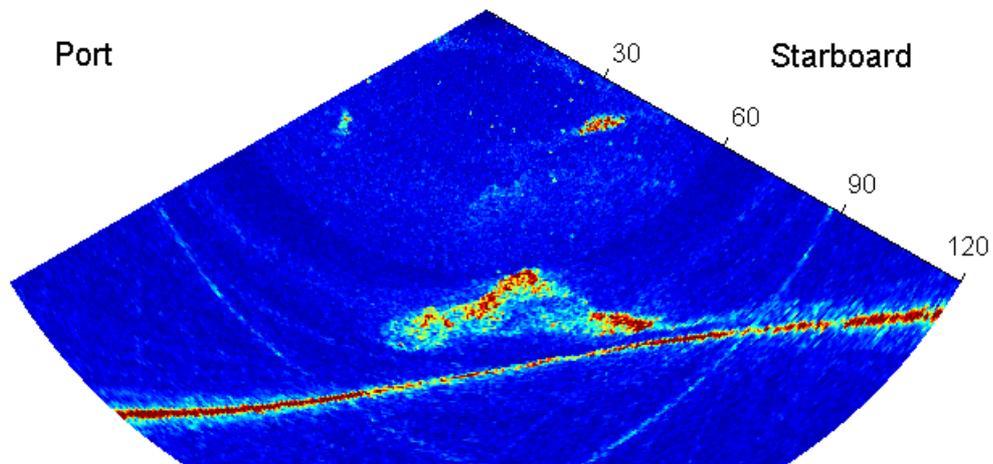
**Figure 2** Multibeam sonar intensity (raw) image, taken at 0912 PST 19 Nov., 2002. Corresponds to time = 245 s in figure 1. Red linear feature sloping upwards from left to right is the seabed. Range in metres.
