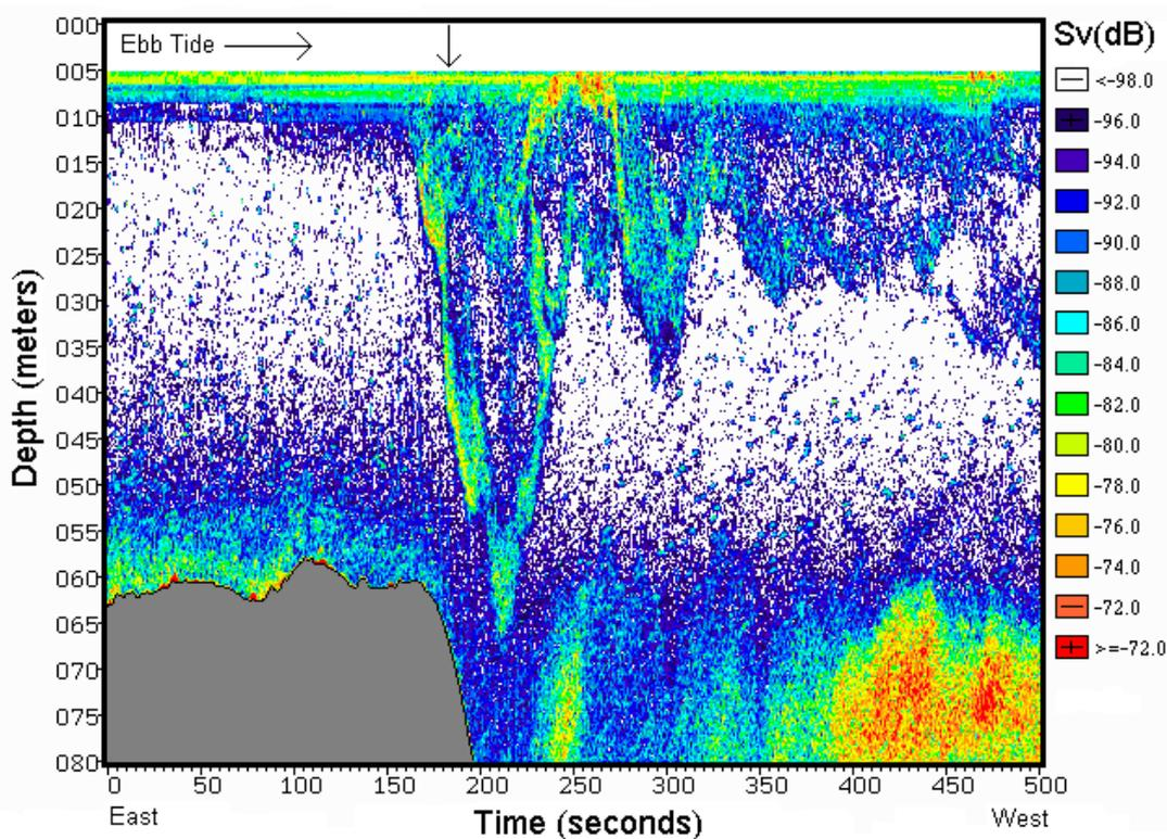
**Figure 5** 120 kHz volume back-scatter vs. depth and time echogram showing microstructure scattering in an internal lee-wave on the western side of the sill. Echogram starts 1421 PST, 17 Nov., 2002, with ship westbound during ebb (westbound) tide. Vertical arrow denotes time of multibeam snapshot shown in Fig. 6.
