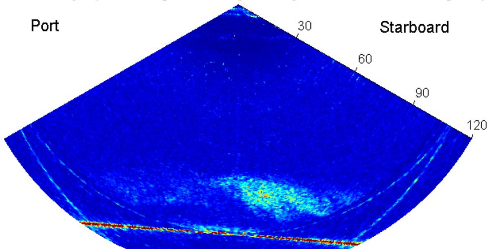
**Figure 4** Multibeam sonar intensity (raw) image, taken at 1114 PST 23 Nov., 2002. Corresponds to time = 85 s in figure 3. Red linear feature sloping downwards from left to right is the seabed. Range in metres.
