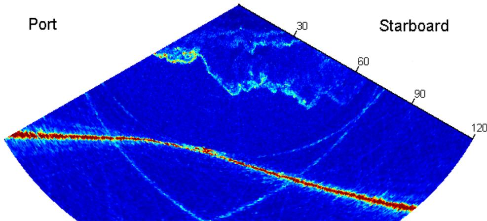
**Figure 6** Multibeam sonar intensity (raw) image, taken at 1424 PST 17 Nov., 2002. Corresponds to time = 185 s in figure 5. Red linear feature sloping downwards from left to right is the seabed. Range in metres.
