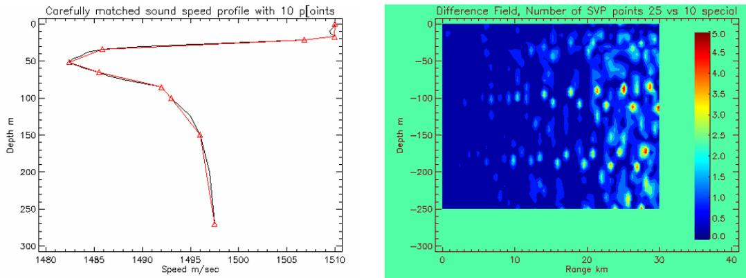
**Figure 14. Left: 10-point speed profile carefully selected to match the 25-point profile at inflection points. Right: TL Difference field at 1500 Hz using the carefully selected profile. Mean error has been reduced from 5.38dB using the automated 10-point profile (see Figure 12) to 0.51 dB using the carefully selected 10-point profile.**
