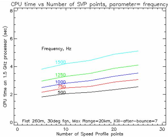
**Figure 16. CPU time vs frequency and number of profile points for a 30°angle fan allowing only 7 bounces. Upper left uses a 25 point SSP, upper right uses a 10 point SSP. Lower graph uses a max range of 20km.**
