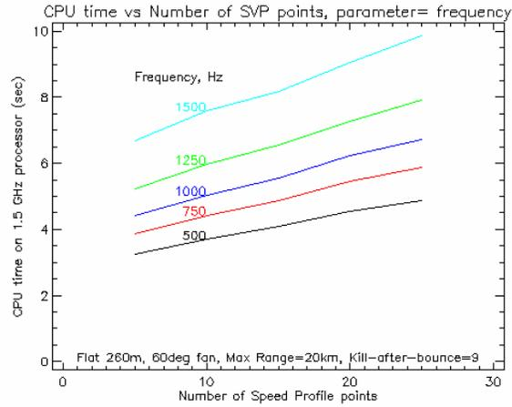
**Figure 15. CPU time vs frequency and number of profile points for a 60°angle fan allowing 9 bounces. Upper left uses a 25 point SSP, upper right uses a 10 point SSP. Lower graph uses a max range of 20km.**
