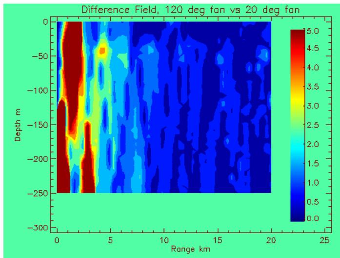
**Figure 7. Comparison of the difference in dB between the full field transmission loss predictions using a 120° angle fan and a 20° angle fan.**
