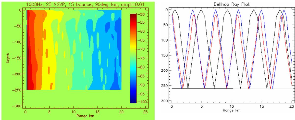
**Figure 2. On the right, three rays are traced from  $-2.5^\circ$ ,  $-0.5^\circ$ , and  $+3.5^\circ$  from a source at 18.3m. On the left, an incoherent acoustic field is plotted for 1000 Hz,  $90^\circ$  angle fan.**
