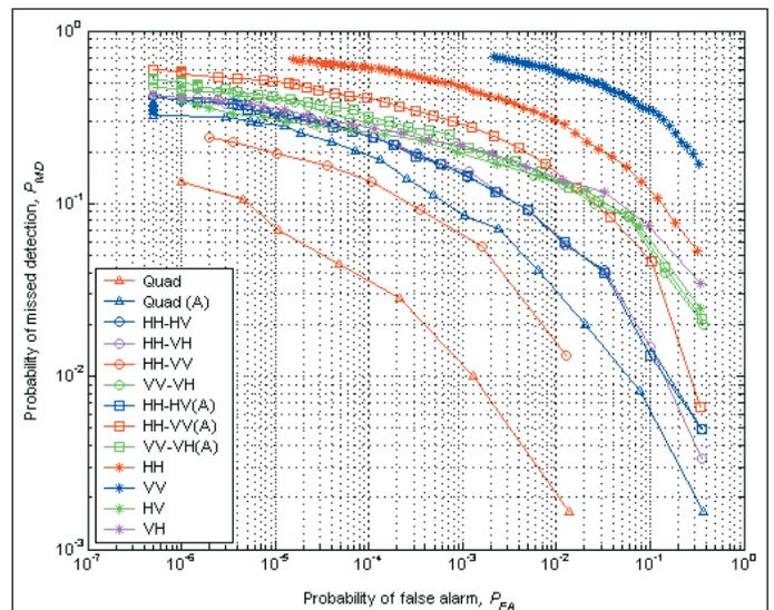
**Figure 3.** Detection performance with ocean statistics only (HMCS *Ville de Québec*, line 3 pass 1, 28 Mar 2000,  $\theta_{inc} = 37^\circ$ , 603 ship pixels,  $2 \times 10^6$  ocean pixels).
