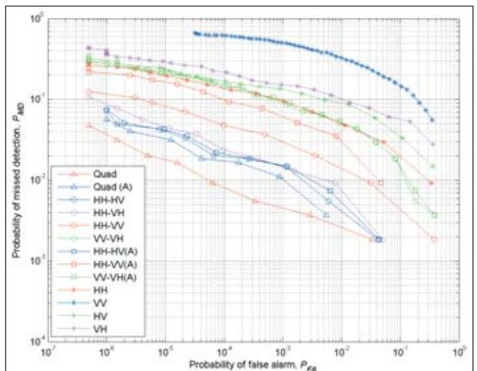
**Figure 7.** Detection performance with ocean statistics only (HMCS *Ville de Québec*, line 5 pass 7, 30 Mar 2000,  $\theta_{inc} = 57^\circ$ , 540 ship pixels,  $2 \times 10^6$  ocean pixels).
