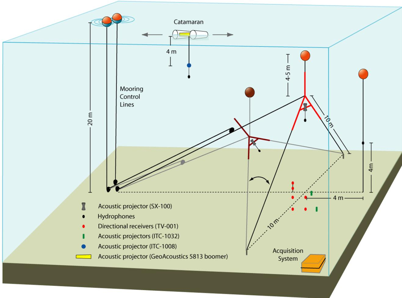
**Figure 1: The experimental geometry to measure sound speed dispersion. Acoustic arrivals are received by sensors buried in the seabed and moored in the water column. There are acoustic sources buried in the seabed, mounted on a catamaran, and in three point moorings (one of two is shown) that can adjust the angle of incidence (grey lines at shallower angle).**
