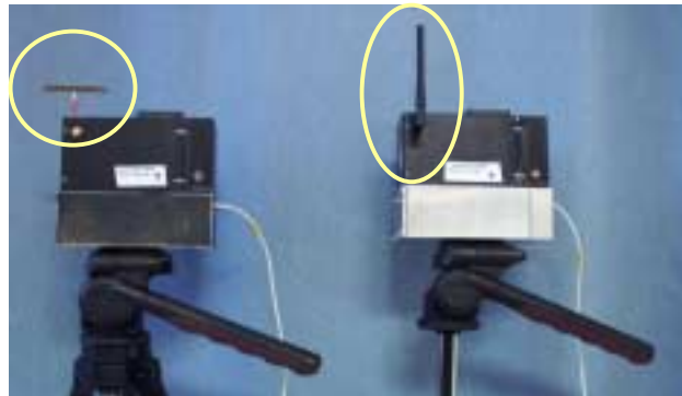
Figure 9. Remote antenna mounting
