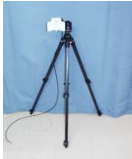
Figure 4. Cirronet 9 dB corner reflector antenna
