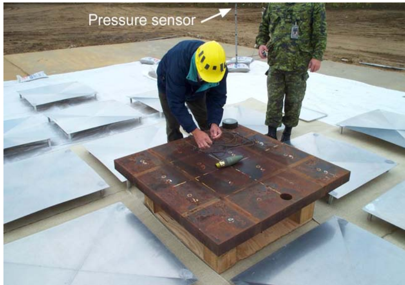
Figure 3. EOD staff installing a detonator on a 60-mm mortar and location of the 5-m pressure sensor
