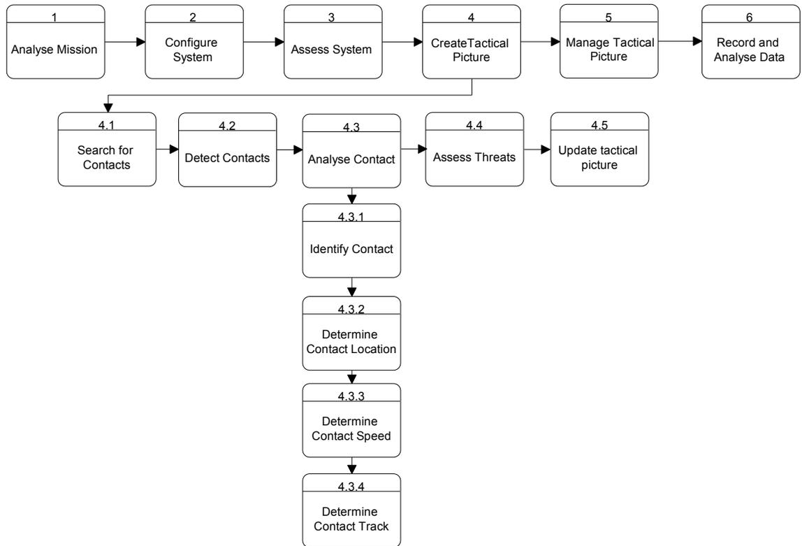
**Figure 1: Function flow diagram of generic sonar system**
