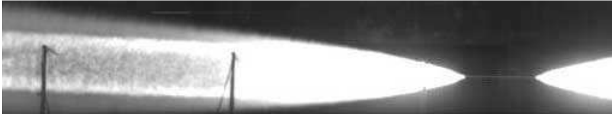
Figure 10 High speed image of detonating cord, initiated on both sides.
