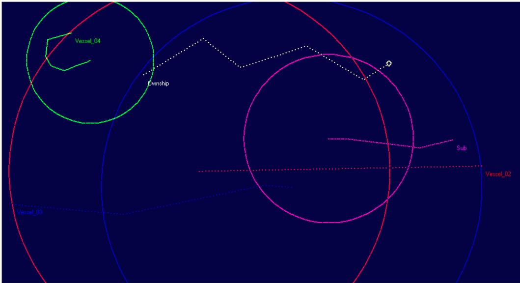
**Figure 10. Target Range Circles for a Single Passive Sensor**
