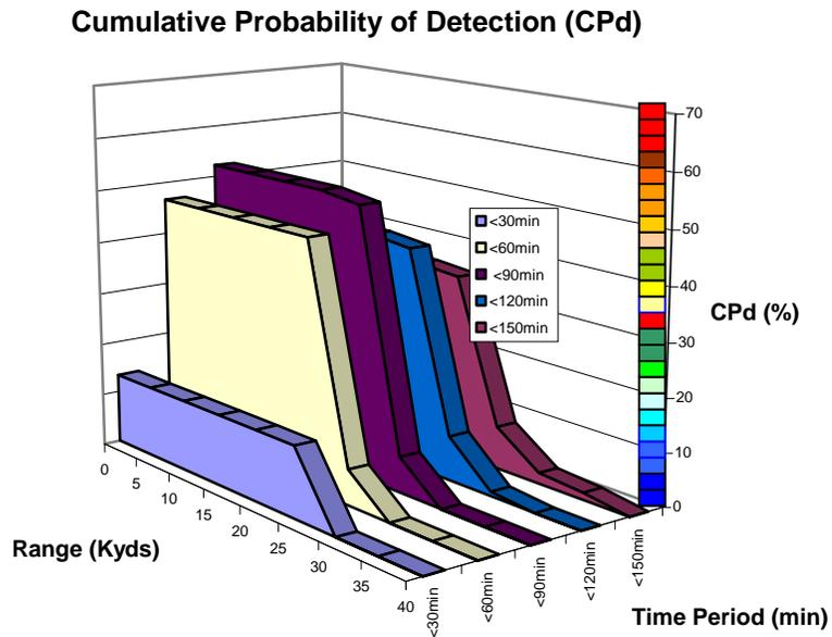
**Figure 9. Example Cumulative Probability of Detection over Increasing Time Periods**
