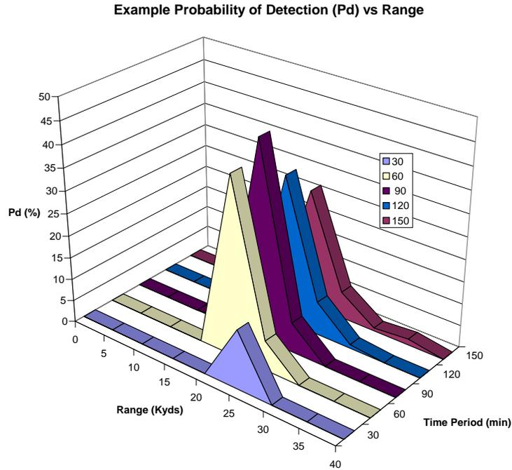
**Figure 8. Example Probability of Detection over Increasing Time Periods**
