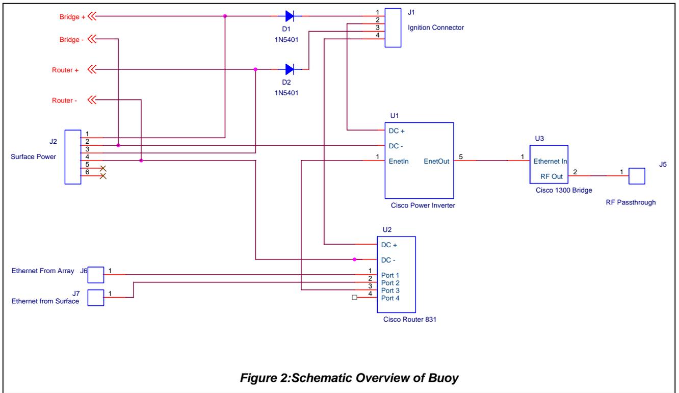
**Figure 2: Schematic Overview of Buoy**
