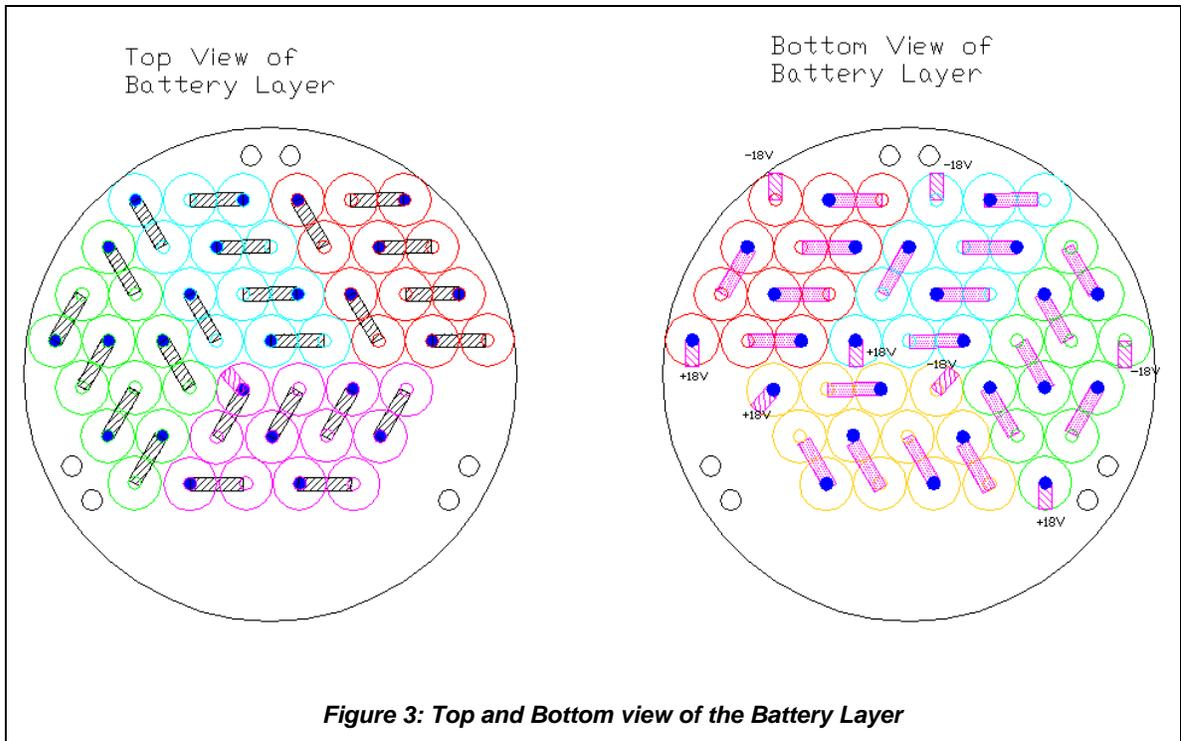
**Figure 3: Top and Bottom view of the Battery Layer**
