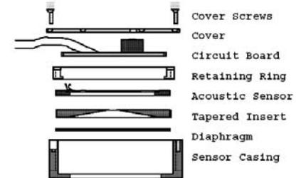
Figure 3: Sensor assembly drawing.
