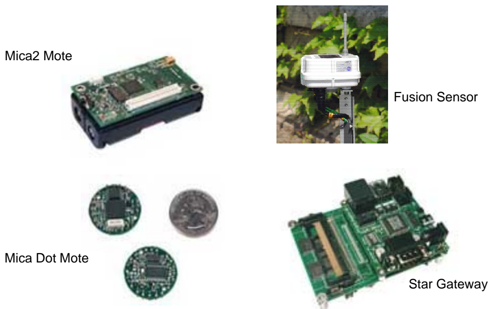
Figure 1: Examples of wireless sensor network nodes
