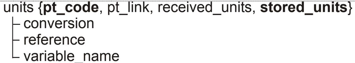
Figure 5. The units brick. This brick contains 4 attributes and three elements. The bold text indicates mandatory content.
