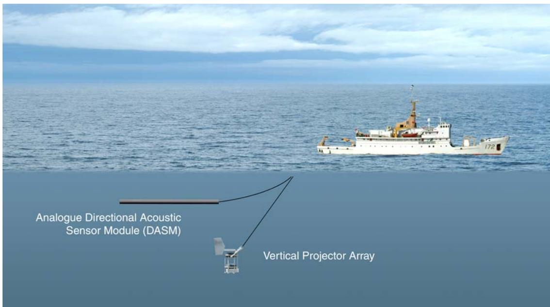
*Fig.1 Cartoon showing tow ship, DASM towed receive array and vertical projector array.*
