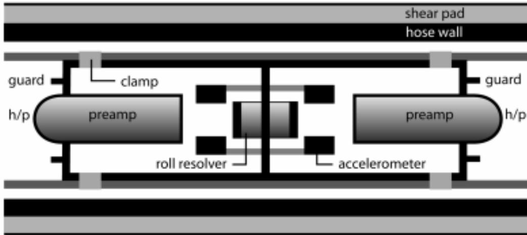
Fig.2 Combined Omni-Roll-resolved Dipole Sensor
