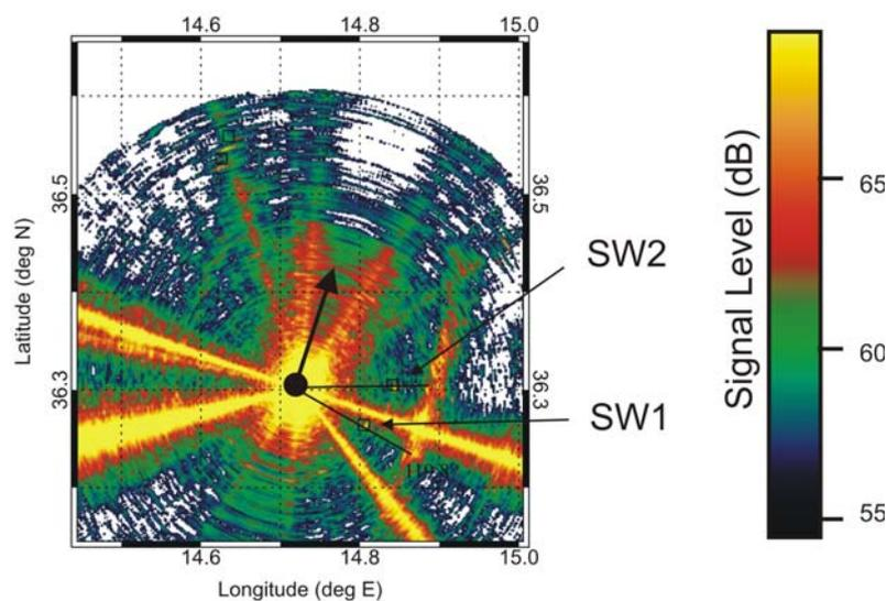
*Fig.3 Plan view showing reverberation map, ship heading (arrow) and wrecks (square boxes) of interest.*
