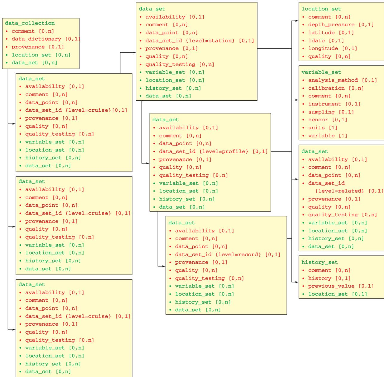
Figure 2. Bricks representing a 1D profile. The green text indicates simple containers, whereas the red text indicates a brick.
