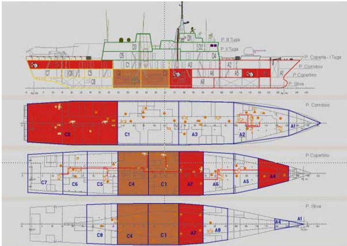
**Figure 1. Screen Shot of ABB Damage Control System.**
