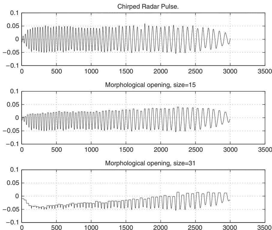
Fig. 1. Morphological opening on a chirped radar pulse.
