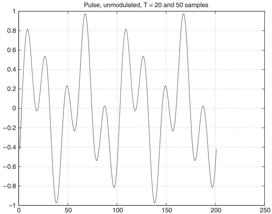
Fig. 6. Pulse fragment, superposition of two tones (period: 20 and 50 samples).
