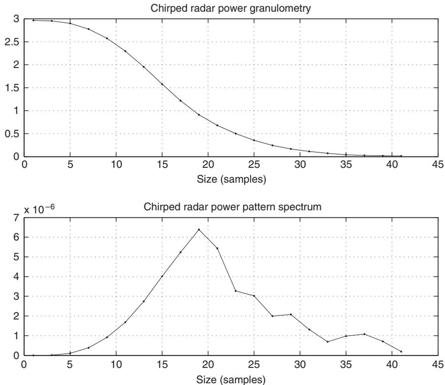
Fig. 8. Power granulometry and power pattern spectrum of a chirped radar pulse.
