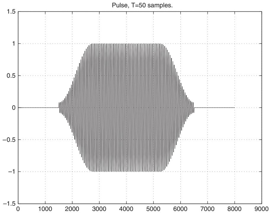
Fig. 3. Simulated radar pulse. Period = 50 samples.
