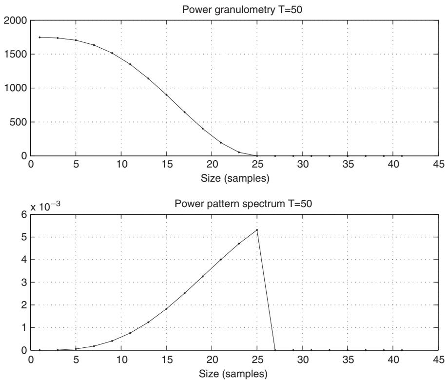
Fig. 4. Power granulometry and power pattern spectrum of a simulated pulse. Period = 50 samples.
