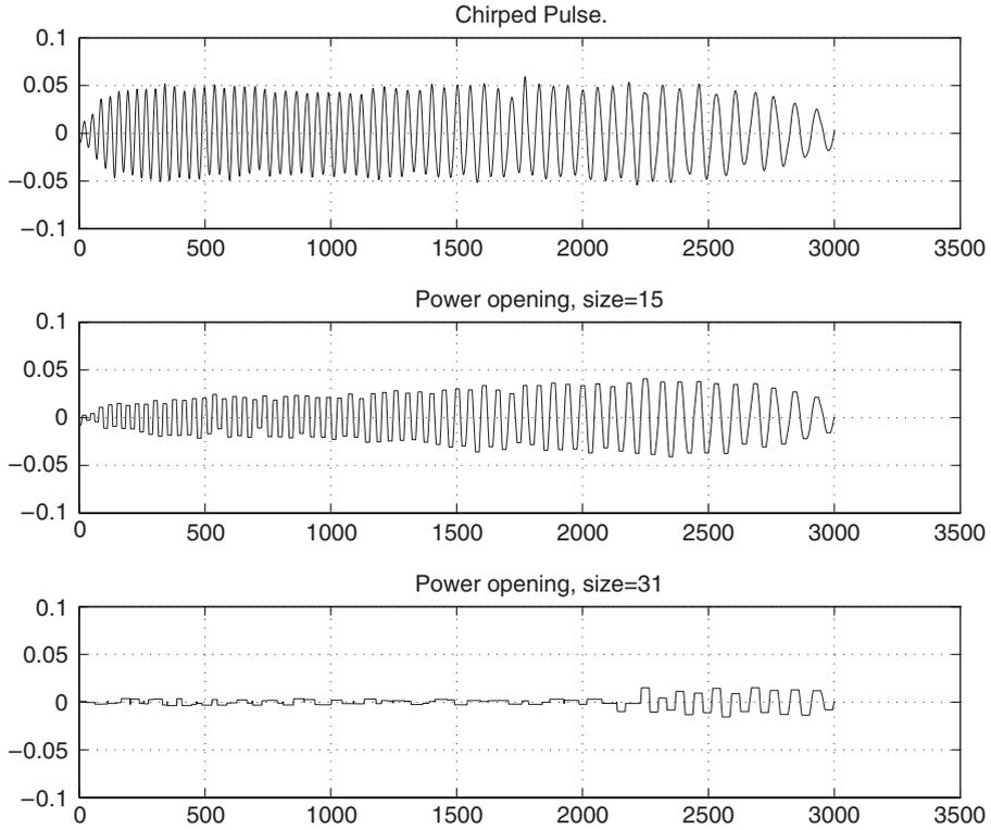
Fig. 2. Complex opening on a chirped radar pulse.
