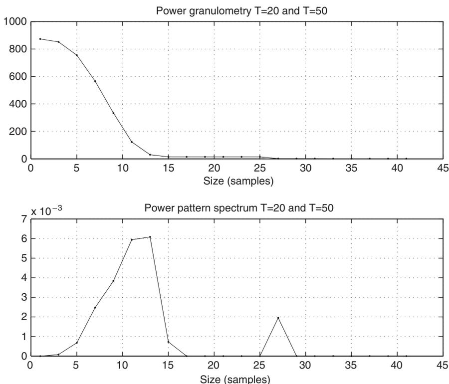
Fig. 7. Power granulometry and power pattern spectrum of a simulated pulse. Superposition of two tones (period: 20 and 50 samples).
