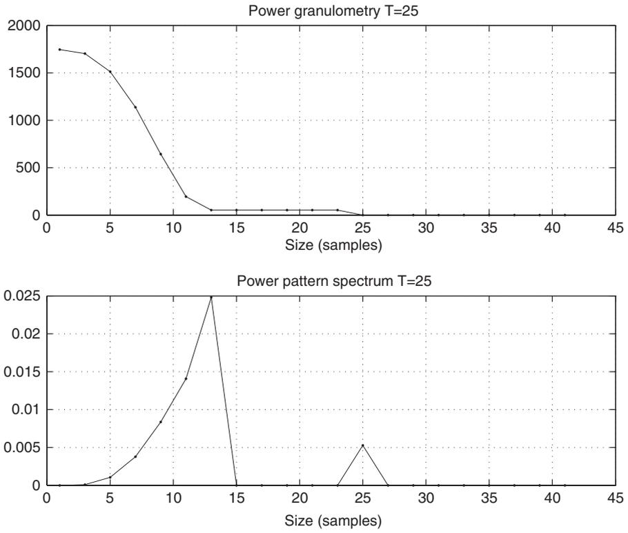
Fig. 5. Power granulometry and power pattern spectrum of a simulated pulse. Period = 25 samples.
