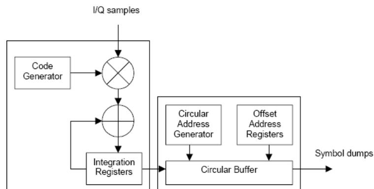
Figure 4.18: Block diagram of the Post-buffer Rake receiver.
