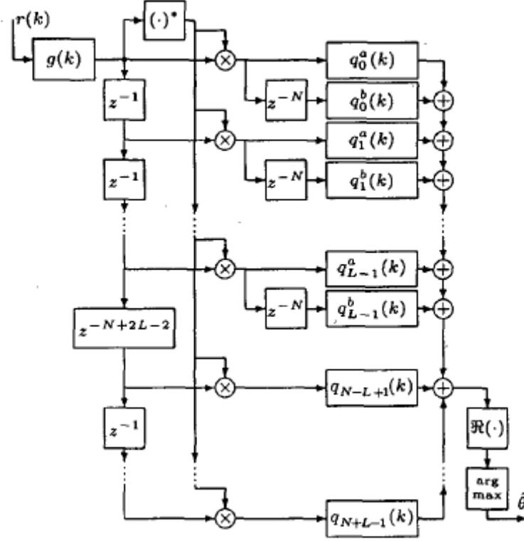
Figure 3.3: Example of the ML estimator structure.
