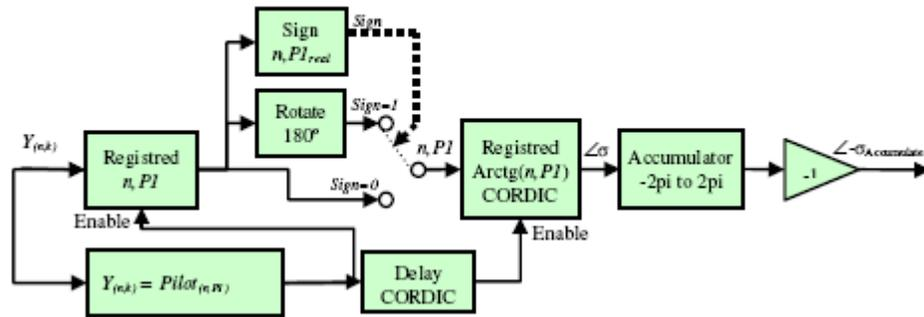
Figure 3.13: Block diagram for phase tracking.
