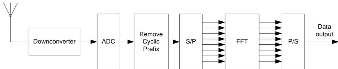
Figure 2.4: Basic blocks of an OFDM receiver.
