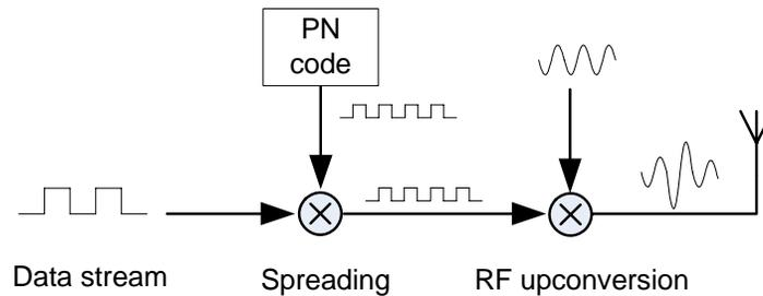
Figure 2.5: Example of a simple CDMA transmitter.
