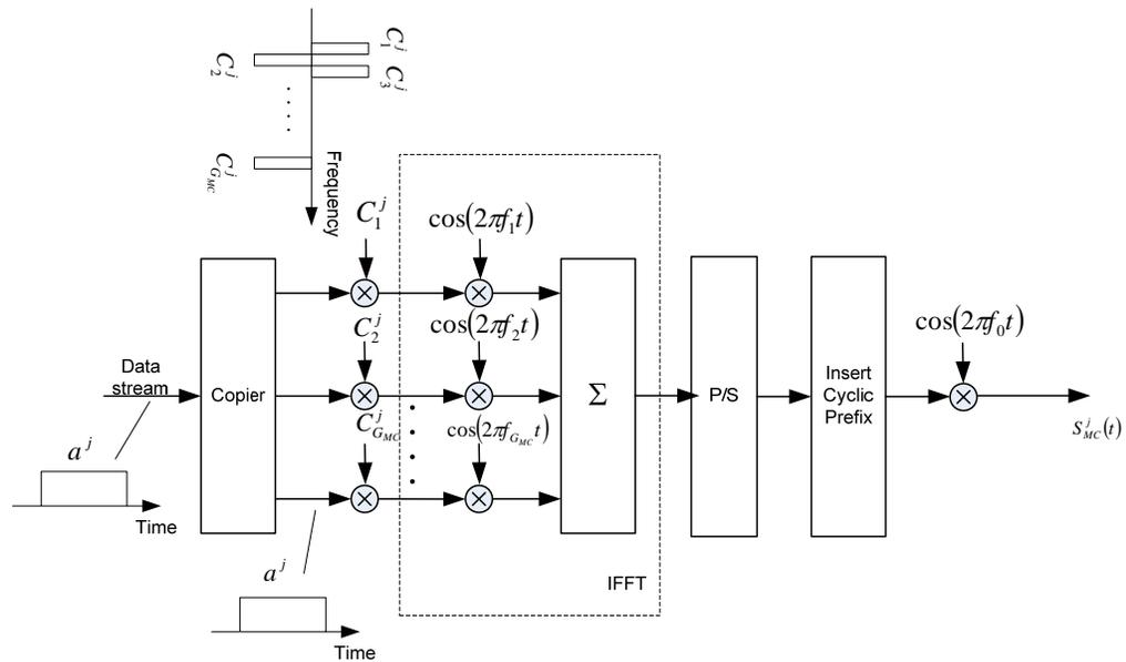
Figure 2.9: MC-CDMA transmitter.
