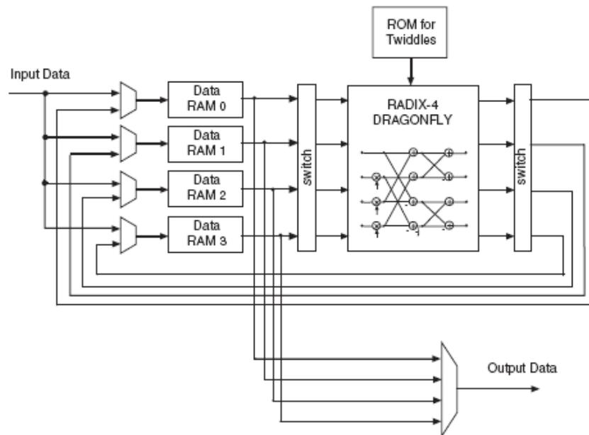
Figure 3.2: Radix-4 burst I/O.
