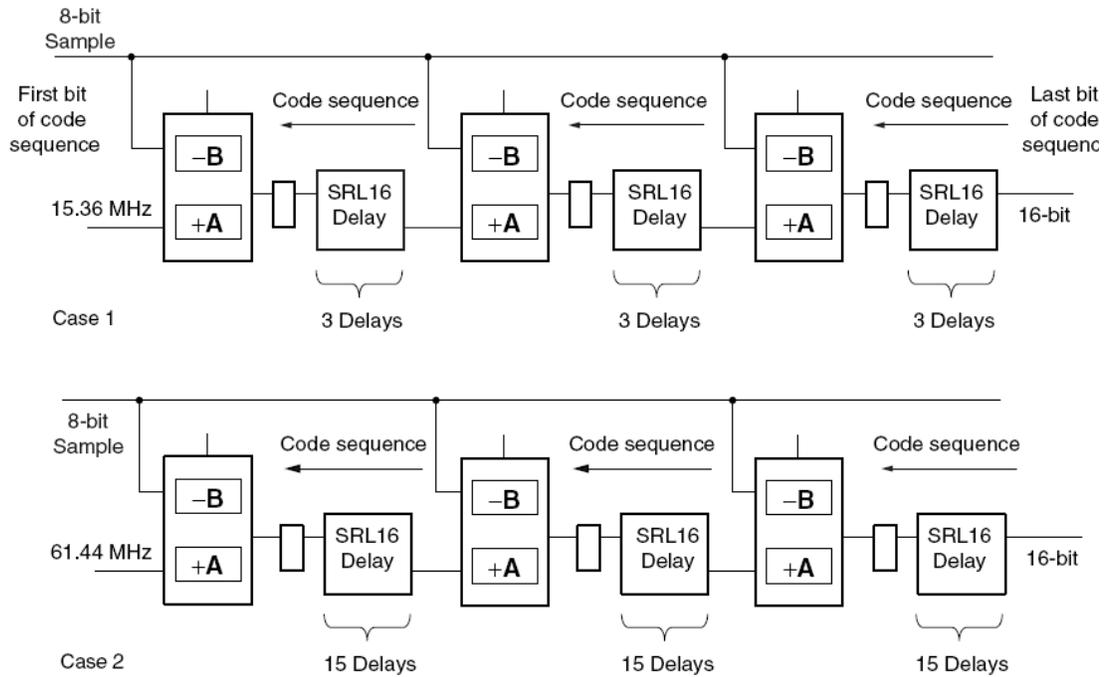
Figure 4.9: Parallel matched filter with 4x and 16x over-sampling.
