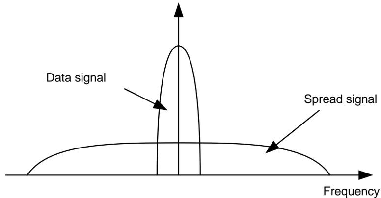
Figure 2.7: Power spectrum of the spread signal versus the data signal.
