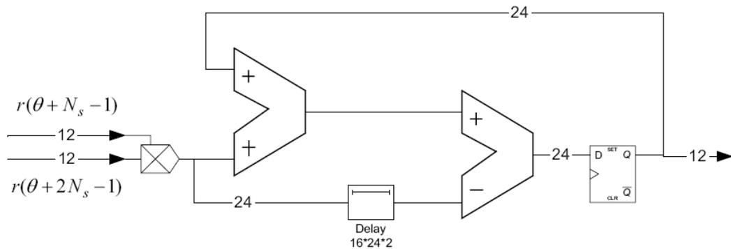
Figure 3.6: Architecture of the correlator using iterative calculations.
