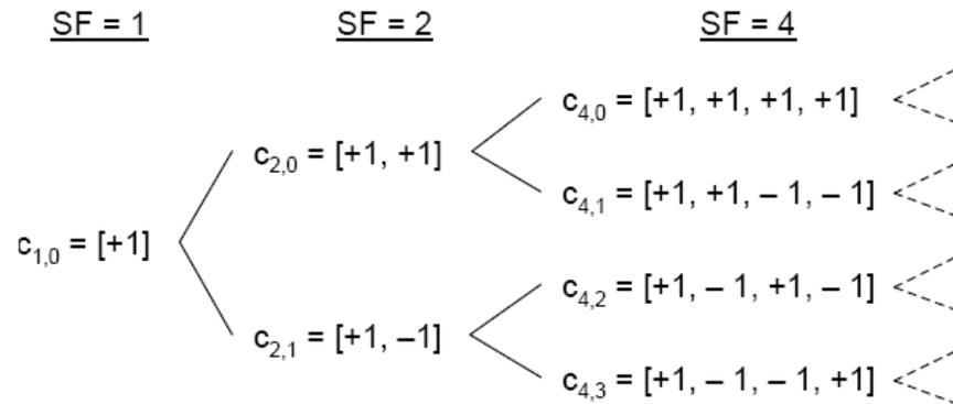
Figure 2.8: Tree structure of the orthogonal variable spreading factor.
