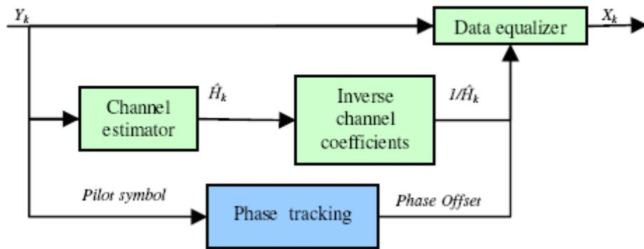
Figure 3.11: Block diagram of the channel equalizer.
