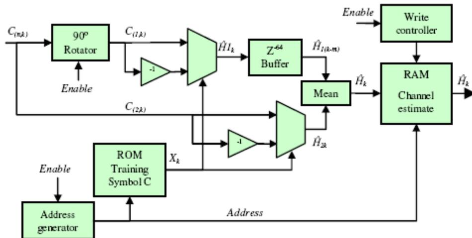
Figure 3.12: Block diagram of the channel estimator.
