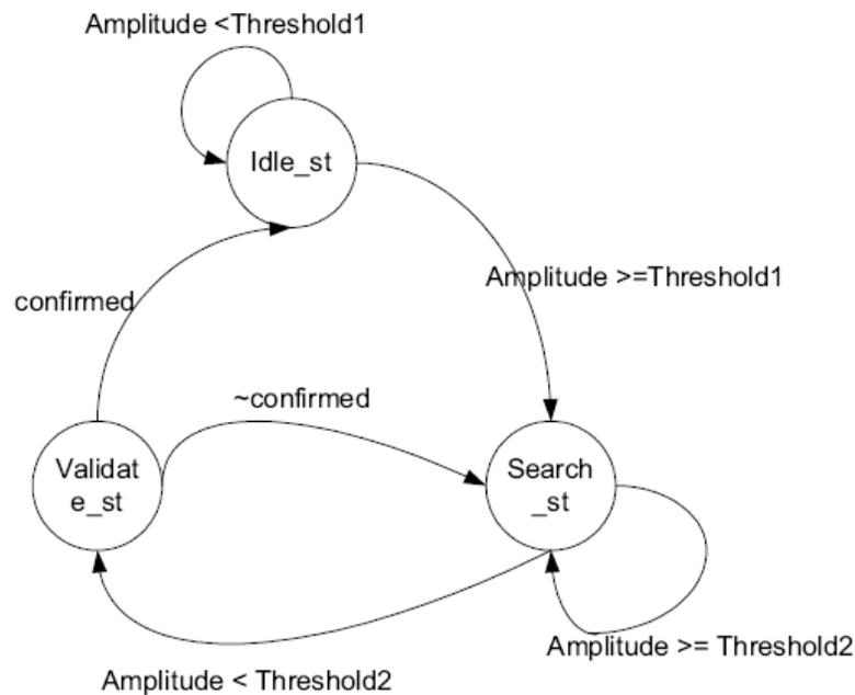
Figure 3.7: State diagram for the peak detector.
