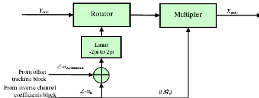
Figure 3.14: Block diagram of the data equalizer.
