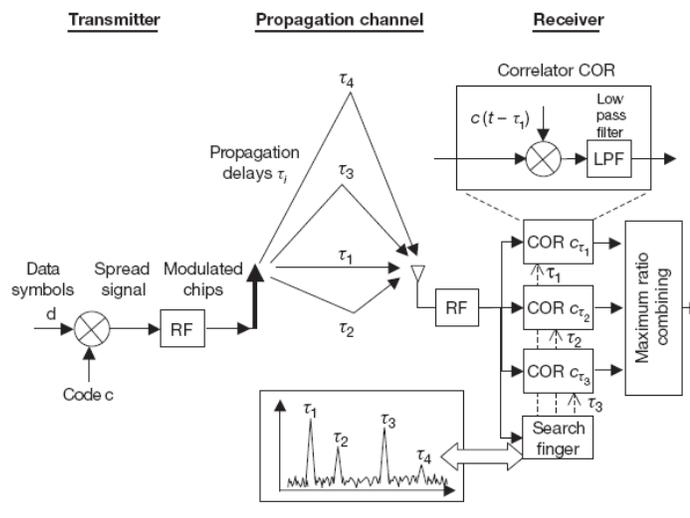
Figure 4.14: Illustration of the RAKE receiver.
