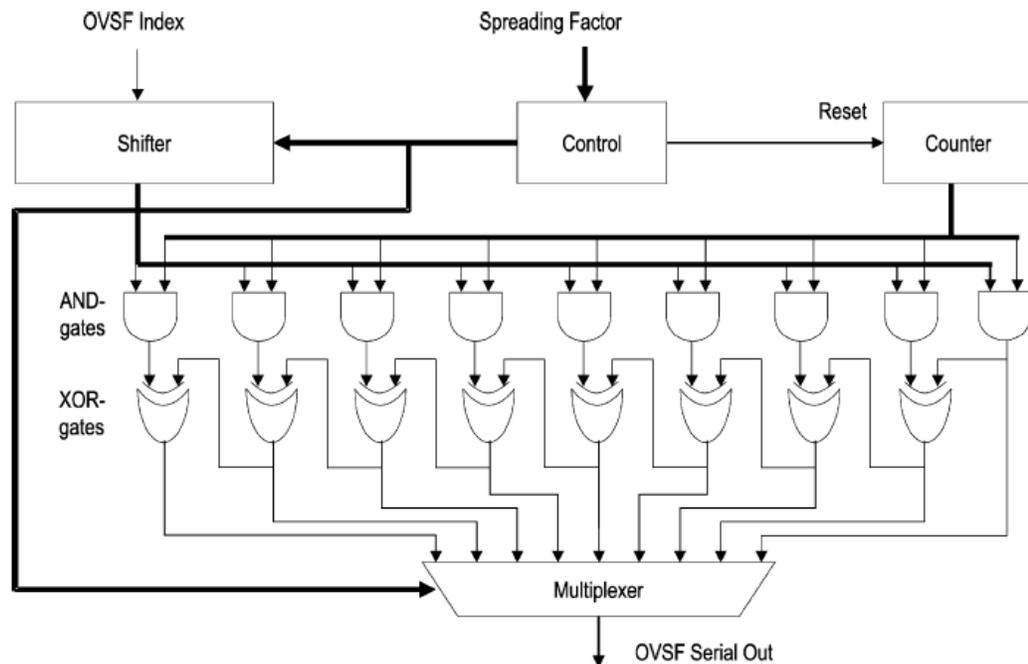
Figure 4.13: OVSF generator architecture.
