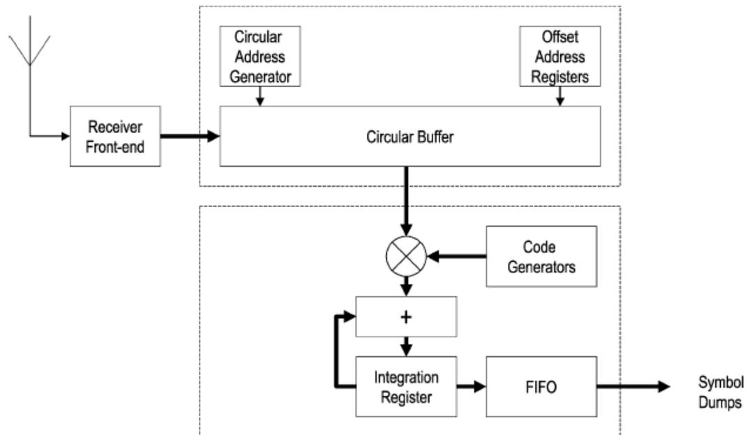
Figure 4.16: Block diagram of the FlexRake receiver.
