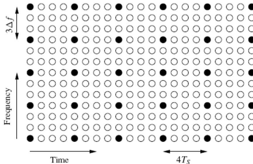
Figure 2.11: Example of a rectangular pilot symbols grid.
