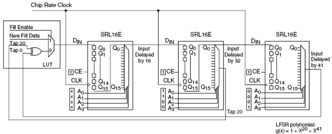
Figure 4.1: 41-stage, 2-tap LFSR with three SRL16s.
