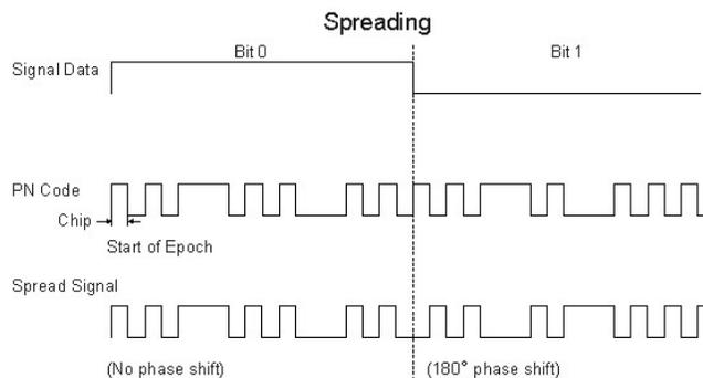
Figure 2.6: Example of the pseudonoise spreading.
