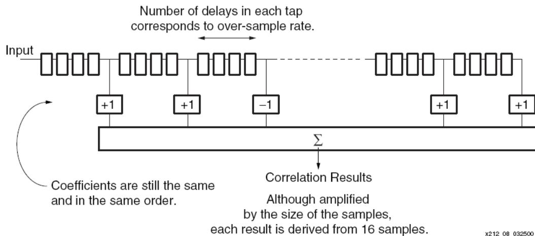
Figure 4.6: Matched filter with a 4x over-sample rate.
