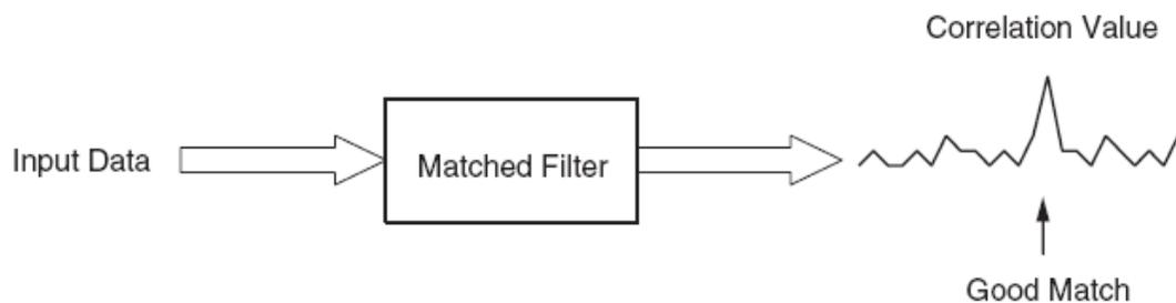
Figure 4.2: CDMA matched filter basic operation.
