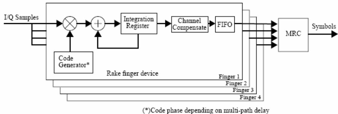
Figure 4.15: Conventional Rake receiver architecture.
