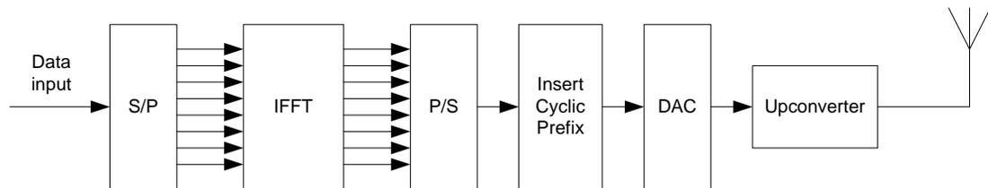
Figure 2.1: Basic blocks of an OFDM transmitter.
