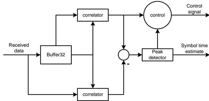
Figure 3.5: Block diagram of the timing estimator.
