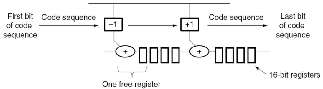
Figure 4.7: Transposed form of the FIR filter with over-sampling.
