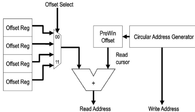
Figure 4.17: Block diagram of the Sample Buffer.
