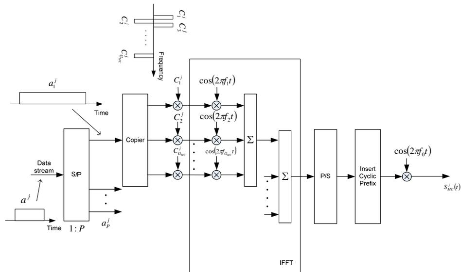
Figure 2.10: Modification of the MC-CDMA transmitter.
