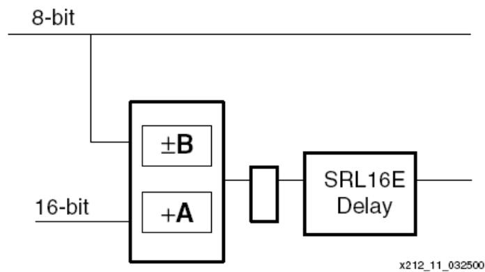
Figure 4.8: Processing element with an SRL16E.
