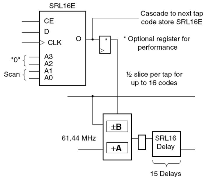
Figure 4.10: Four different code sequences applied to the control pin of a processing element.
