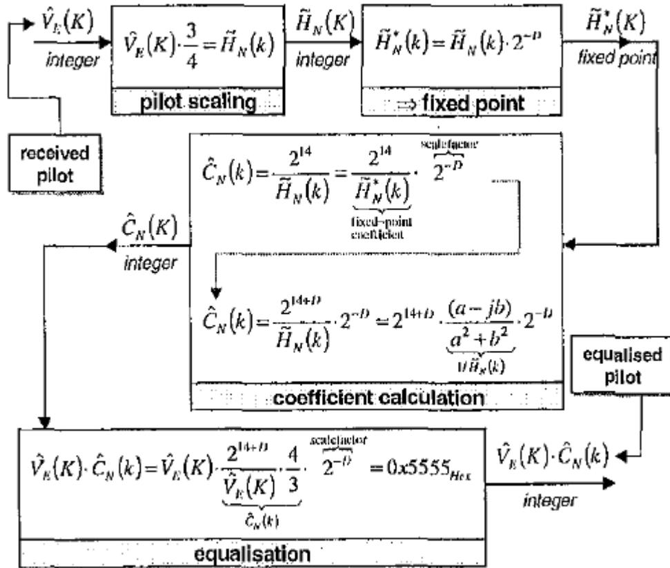
Figure 3.10: Flowchart for pilot equalization using fixed point coefficients.
