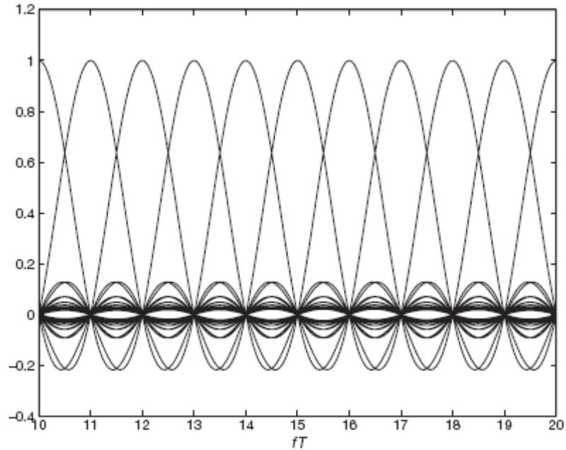
Figure 2.2: Orthogonal overlapping spectral shapes for OFDM.
