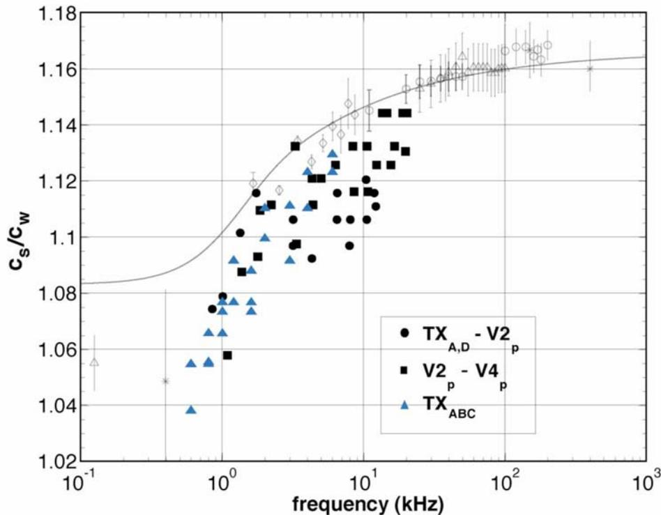
**Figure 3:** A comparison of sound speed measurement during SAX04 (solid symbols) using the time-of-flight technique (Hines *et al.*, 2005b), including vertical and horizontal propagation paths between sources and receivers, with the results from SAX99 (hollow symbols) (Williams *et al.*, 2002).
