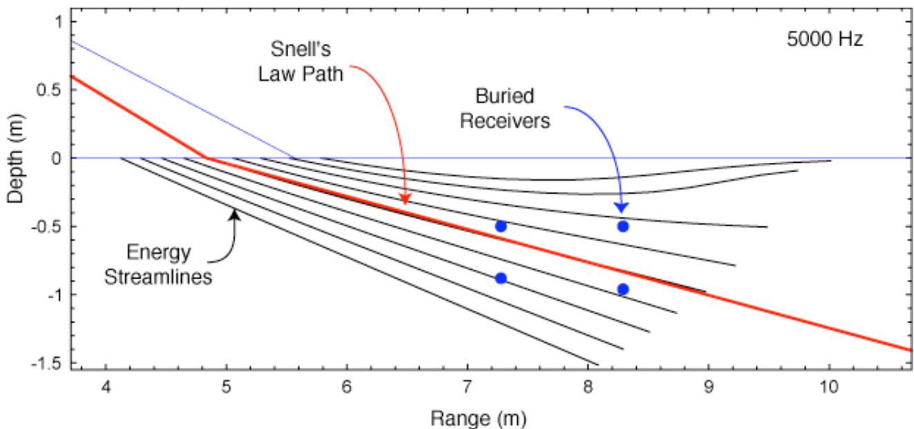
**Figure 2: Energy flux streamlines into the seabed (black lines) for an acoustic arrival at 5 kHz just above the critical grazing angle (blue line). One application of this simulation is to determine the sensor positions (blue dots), frequencies and grazing angles at which Snell's Law (red ray path) is valid and when it is not because of the influence of inhomogeneous waves.**
