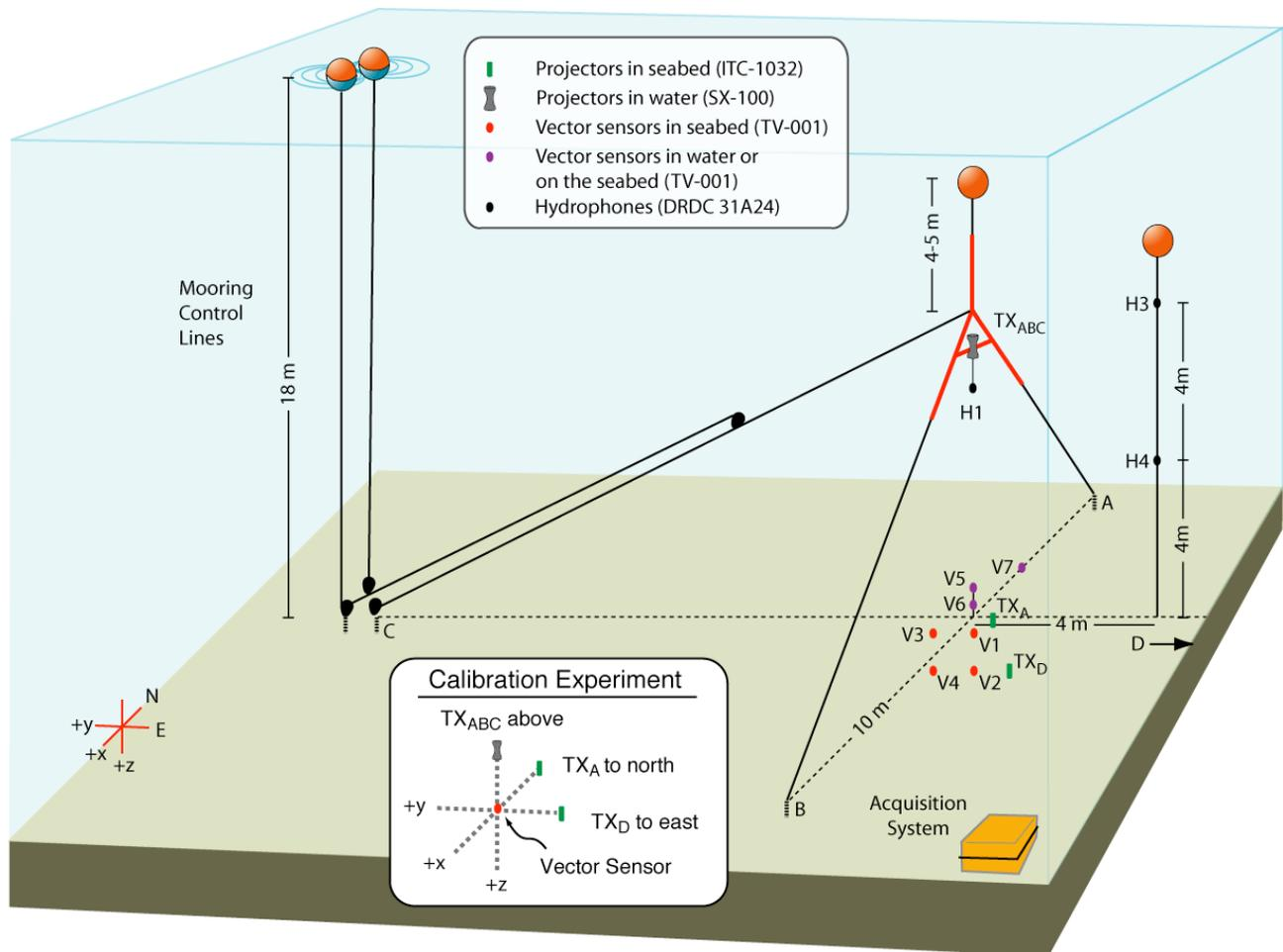
**Figure 1: The experimental geometry to measure sound speed dispersion. Acoustic arrivals are received by sensors buried in the seabed and moored in the water column. There are acoustic sources buried in the seabed and in three point moorings (one of two is shown) that can adjust the angle of incidence.**
