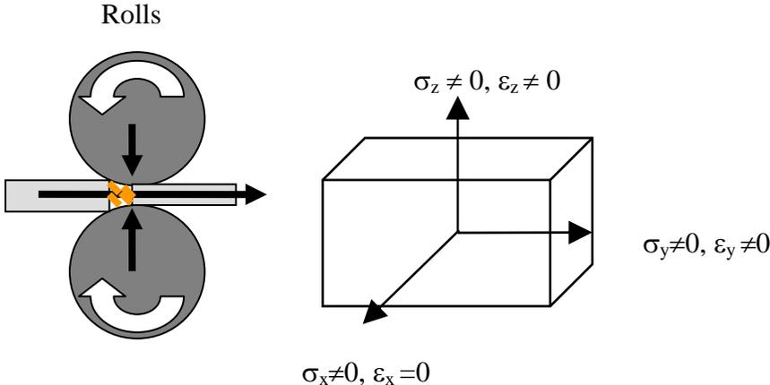
Figure 4. Plane strain compression during rolling.
