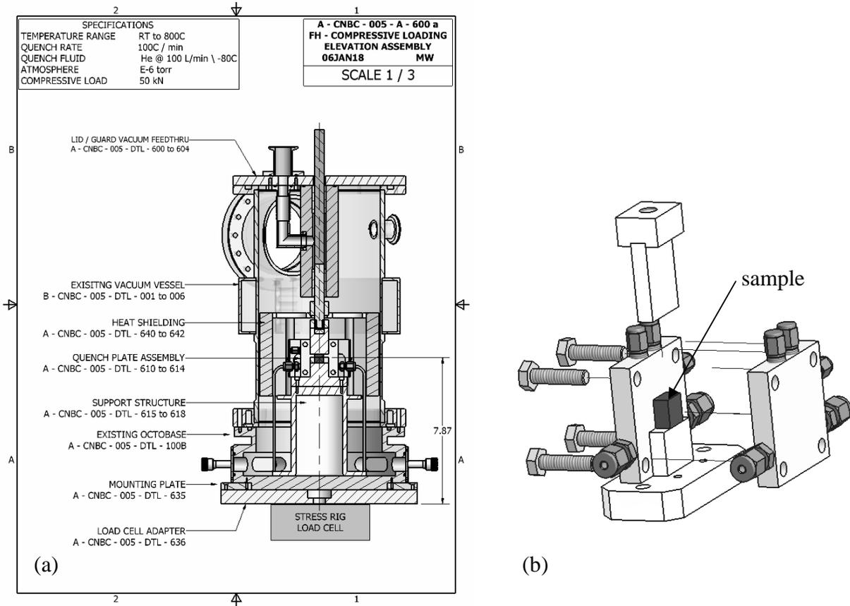
**Figure 5.** Schematics of (a) the compressive loading furnace assembly (not to scale) and (b) the channel-die compression assembly at the Canadian Neutron Beam Centre. The die walls will have embedded channels for cooling fluid to provide cooling rates of about 50 K/min.
