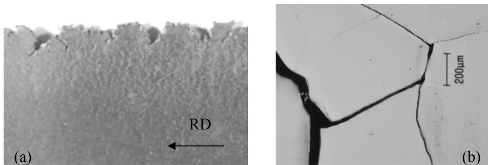
Fig. 3. (a) Edge cracking on hot rolled specimen after about 80% reduction; (b) optical micrograph of as-rolled specimen showing grain boundary fracture.
