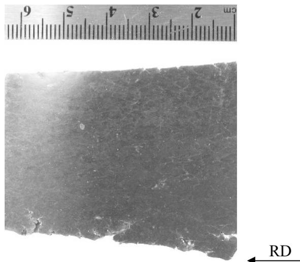
Fig. 6. A Galfenol specimen after warm rolling to a thickness of about 0.5 mm.
