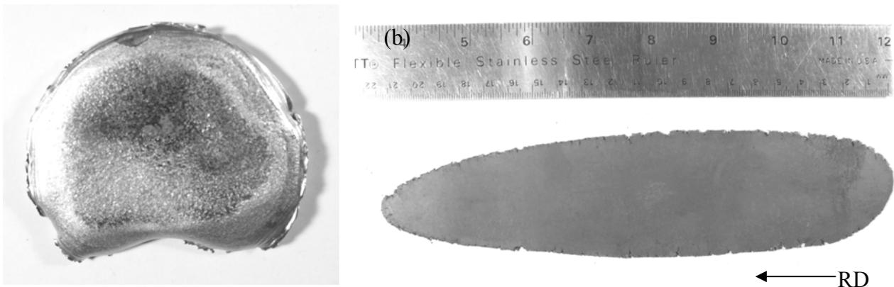
Fig. 2. (a) Galfenol arc-melted button (18.4at% Ga) used as starting material for hot rolling, (b) same specimen after hot rolling with about 80% reduction.
