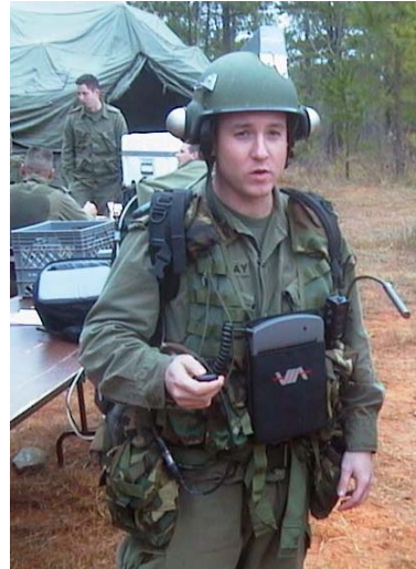
Figure 8: Land Warrior tablet worn with audio FIND system
