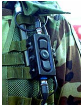
Figure 3: Land Warrior central processor and mouse
