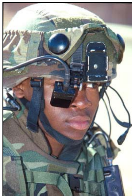
Figure 6: US Land Warrior Helmet Mounted Display (HMD)
