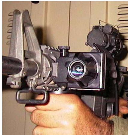
**Figure 4: Weapon Mounted Daylight Video Sight (Front)**
