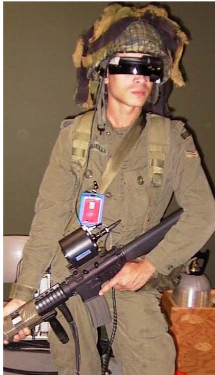
**Figure 6: The DCIEM Helmet Mounted Gunsight**
