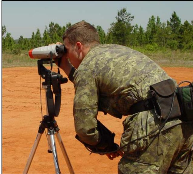
**Figure 2: Soldier using Leica Laser Rangefinder with Digital Map System**
