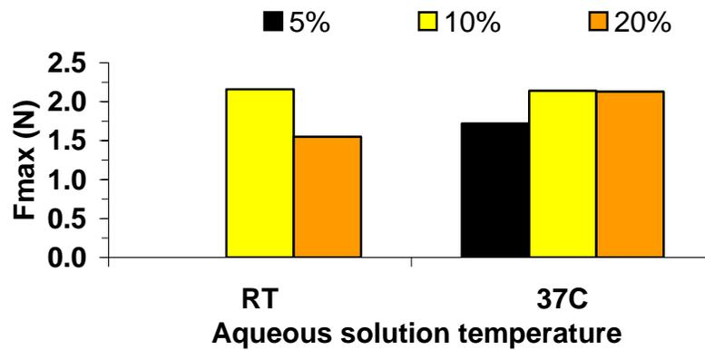
**Figure 10.** Strength of gelatin-HydroThane™ films (prepared with varying amounts of photoinitiator) after a 4-d washing period in distilled water maintained at either room temperature (RT) or 37°C. Data represent n=1 per group.
