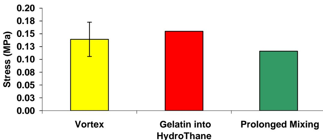
**Figure 12.** Breaking stress of photo cross-linked gelatin-HydroThane™ IPN films re-hydrated for 2 days in serum maintained at 37°C. Three different methods were used for mixing the polymers in the pre-IPN mixture. Data represent n=1 per experimental group except for Vortex (means ± SEM; n=3).
