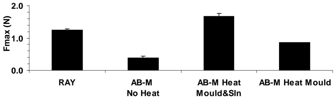
**Figure 16.** Strength of gelatin-HydroThane™ films photo cross-linked in the Rayonet (RAY) or AB-M reactor. Strength was measured after a 4-d immersion in 1% sodium azide aqueous solution. The mould and/or pre-IPN mixtures were pre-warmed for 30 min at 50°C prior to the irradiation procedures. Data represent means  $\pm$  SD, n=3 per experimental condition, except for ABM Heat Mould (n=2).
