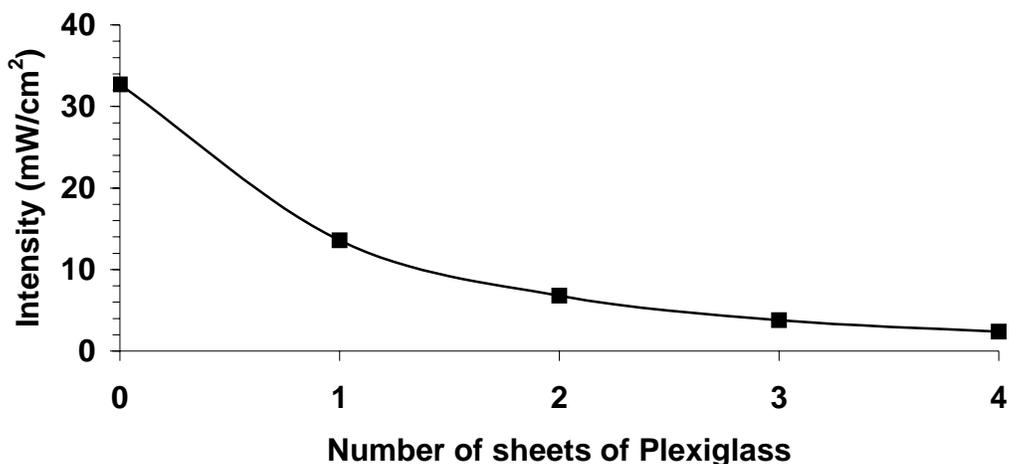
*Figure 17. Relationship between the intensity output of the AB-M reactor and the number of sheets of Plexiglas<sup>®</sup> covering the UV light.*
