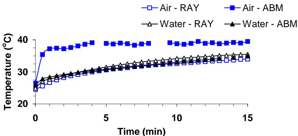
**Figure 14.** Changes in ambient temperature in the chamber of the Rayonet (RAY) and AB-M reactors (ABM) during a 15-min irradiation period of a 2-mL sample of water. Data represent  $n=1$  per experimental condition.
