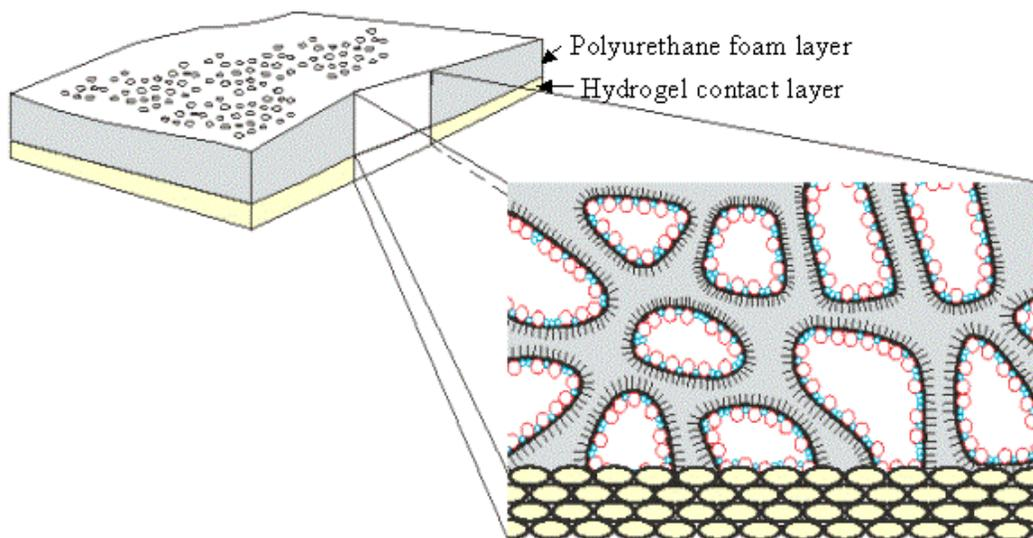
**Figure 1.** Schematic representation of the DRDC bi-layer wound dressing, consisting of a medicated polyurethane foam over a thin tissue-contacting hydrogel layer to reduce adhesion to the wound. Colored circles represent two types of drug loaded in the pores of the foam layer. For the sake of clarity, no drug was represented in the hydrogel layer.
