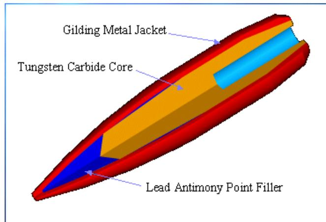
**Figure 1.** Sectioned AP T-C44 projectile
