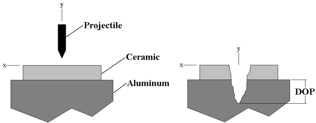
*Figure 3. Depth of penetration testing*
