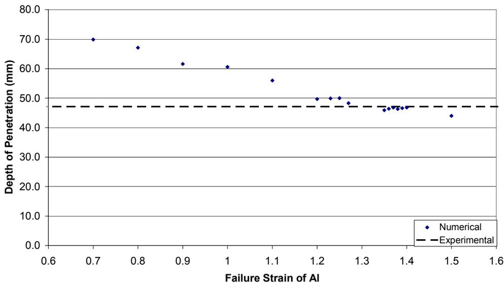
Figure 6. DOP versus failure strain of aluminium target @ 556 m/s
