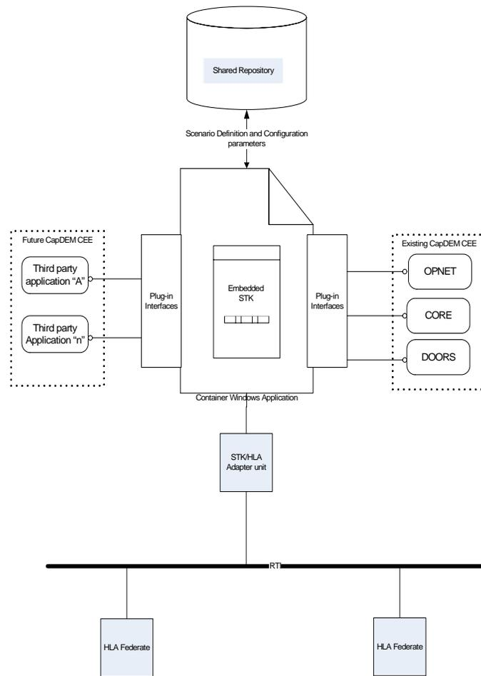
**Figure 7.** “To-Be” Integrated Visualization Architecture
