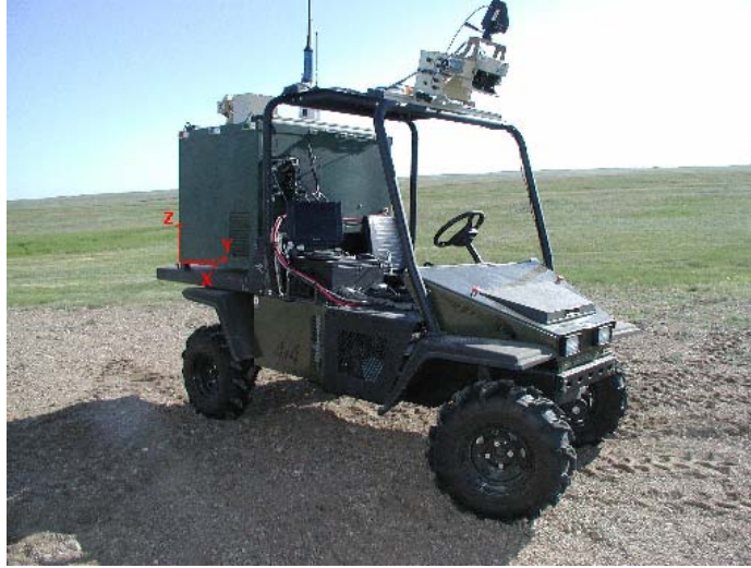
Figure 15: World coordinate system on the Raptor body
