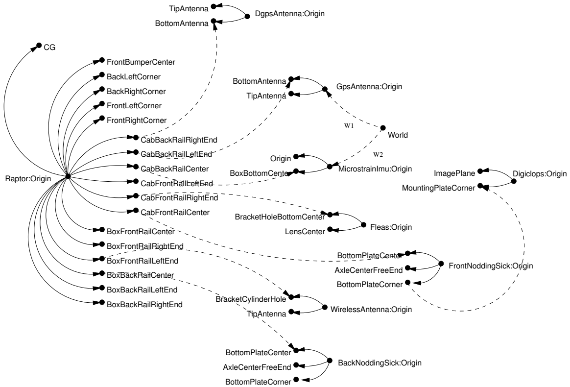
Figure 2: A hierarchical rigid body model.
