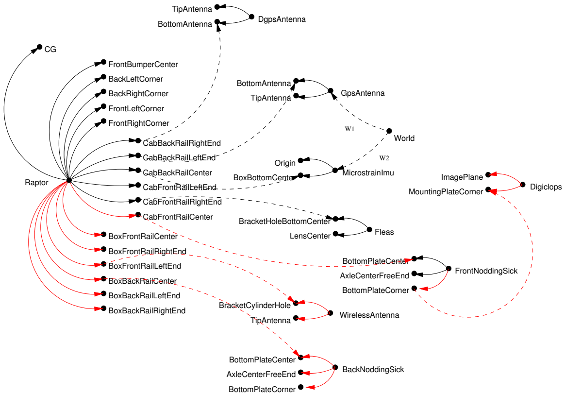
Figure 9: A Depth first search example superimposed in red on DRDC's model tree. With the digiclops imageplane as the frame of interest and the raptor origin as the frame of reference, this figure assumes the search order is bottom to top.
