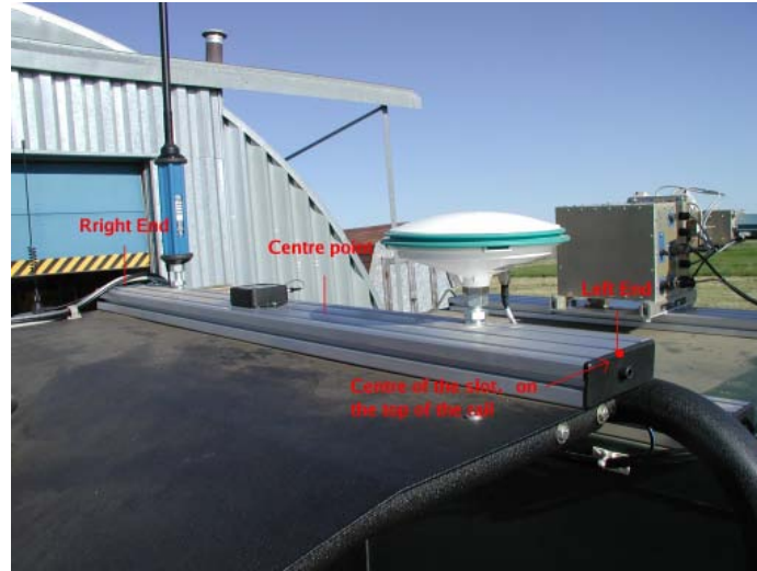
Figure 17: Rail measurement points
