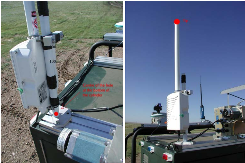
Figure 23: Wireless antenna measurement points
