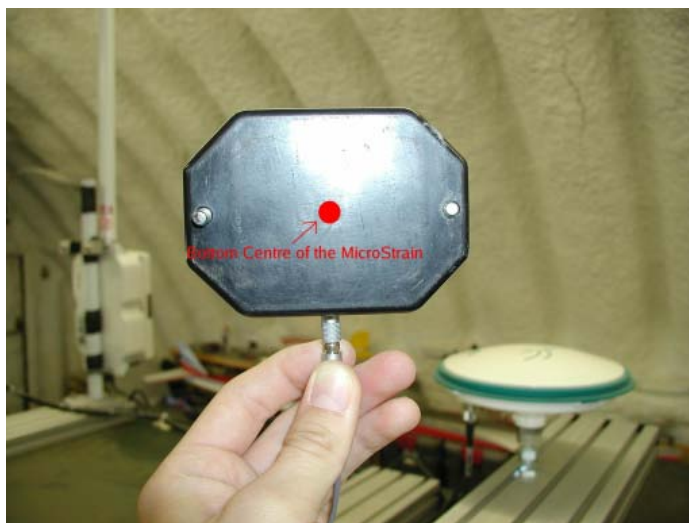
Figure 22: Microstrain IMU measurement point
