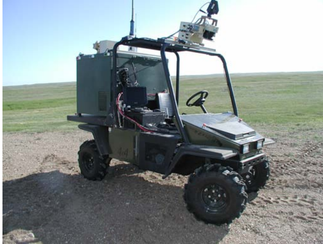
Figure 23: Raptor UGV with Nodding SICK Laser
