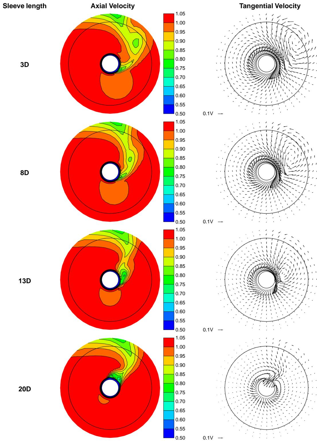
Figure 4: Inflow to the propeller disk with sleeves of different length:  $\Omega = -0.6$ ;  $\alpha = 6^\circ$ ;  $\beta = 10^\circ$ .
