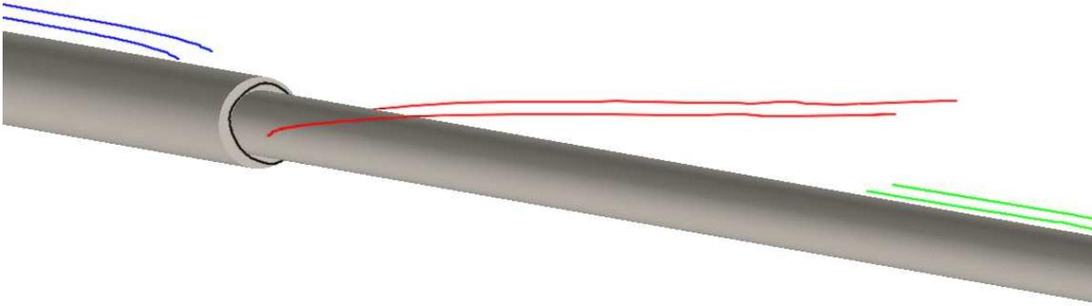
Figure 5: The cores of the principal vortices for a non-rotating shaft with a  $0.2D$  lip
