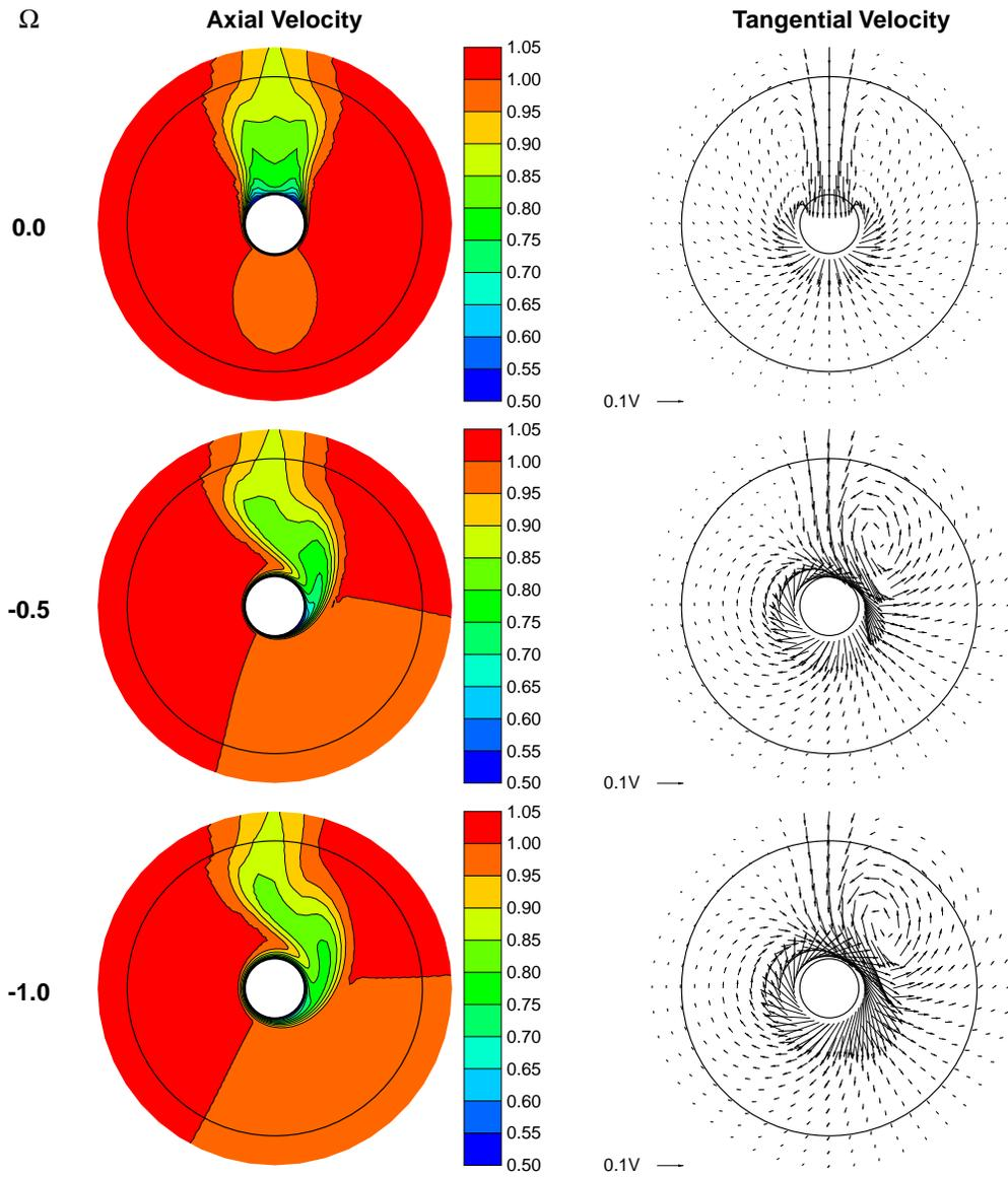
Figure 8: Inflow to the propeller disk at different rotation rates:  $x = 15.8D$ ;  $s = 0.2D$ .
