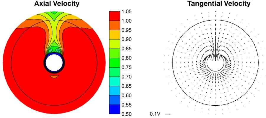
Figure 2: Inflow to the propeller disk with no rotation and no cross-flow
