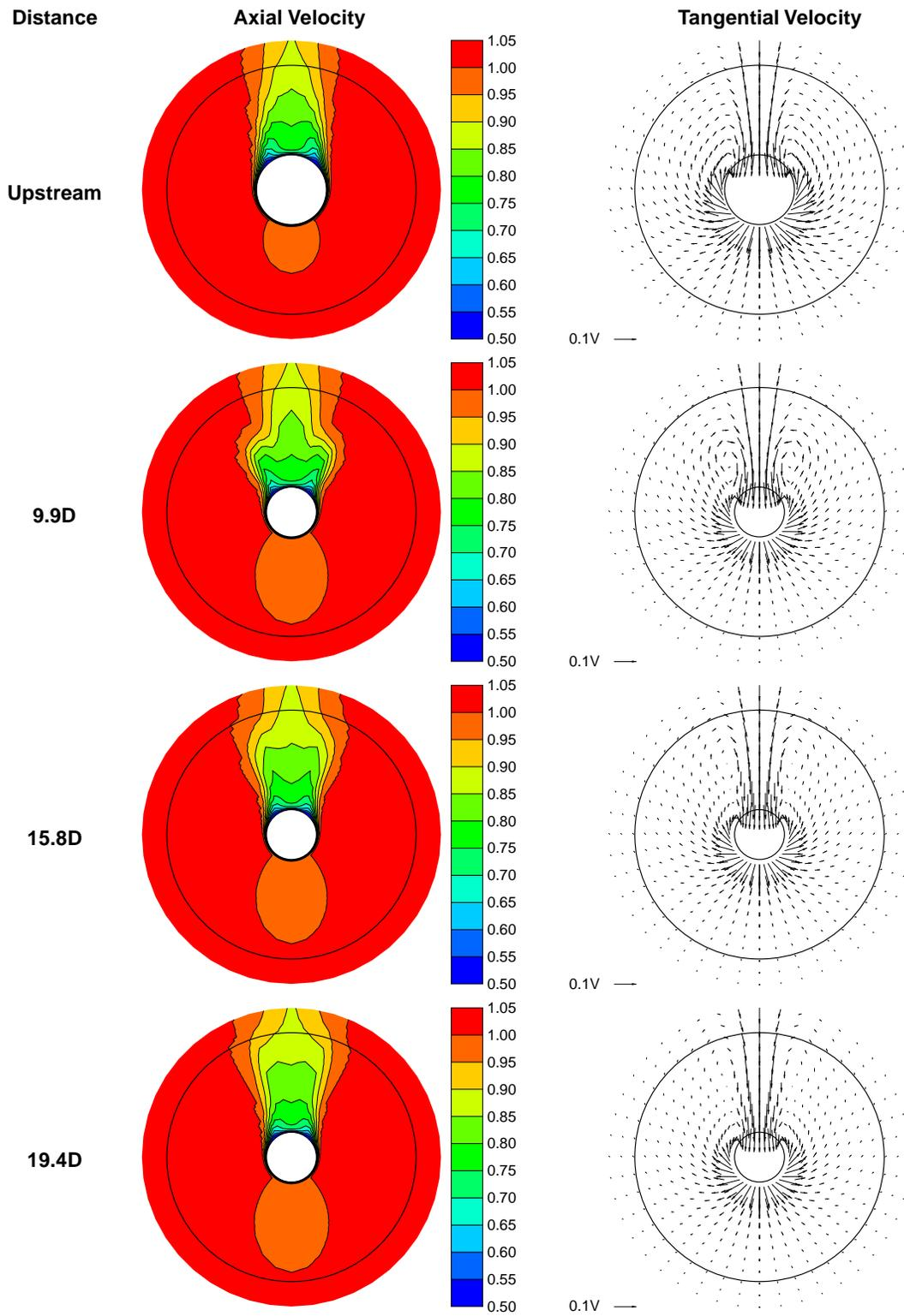
Figure 7: Inflow to the propeller disk at different distances from the lip: no rotation;  $s = 0.2D$ .
