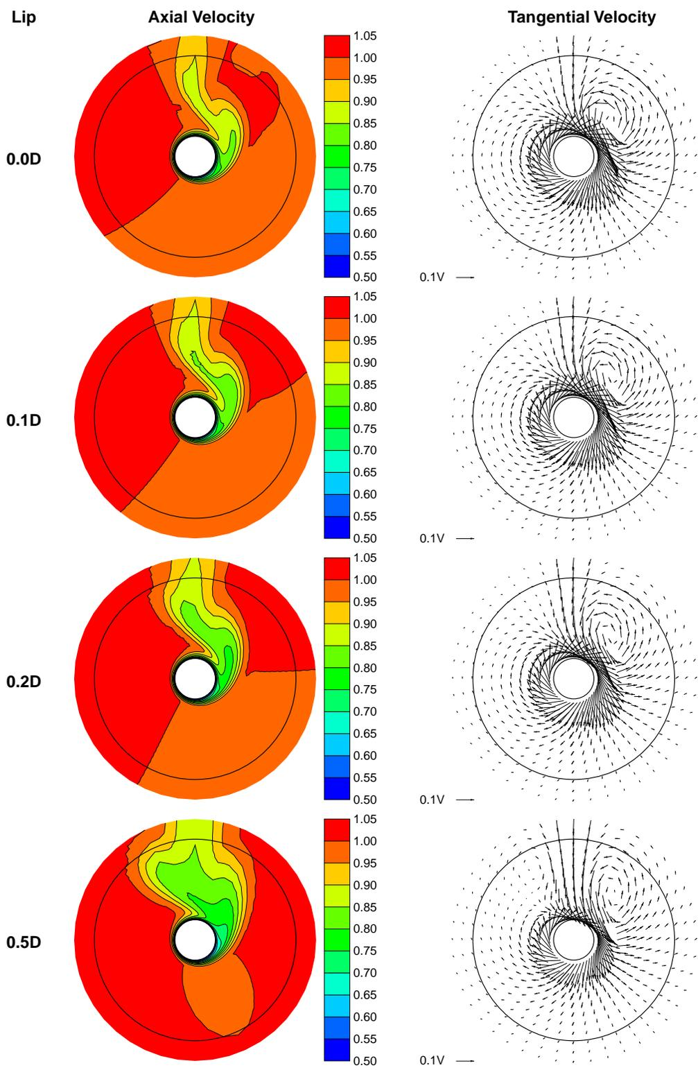
Figure 9: Inflow to the propeller disk for different lip sizes:  $x = 15.8D$ ;  $\Omega = -1.0$ .
