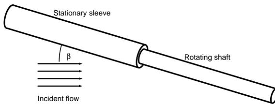
Figure 6: The infinite shaft with a sleeve
