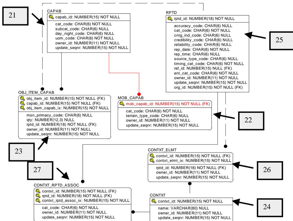
**Figure 3.** The final illustration shows six new tables (RPTD is repeated from Figure 1). These tables describe the capability of the contact and identify that the contact is based on fused information.
