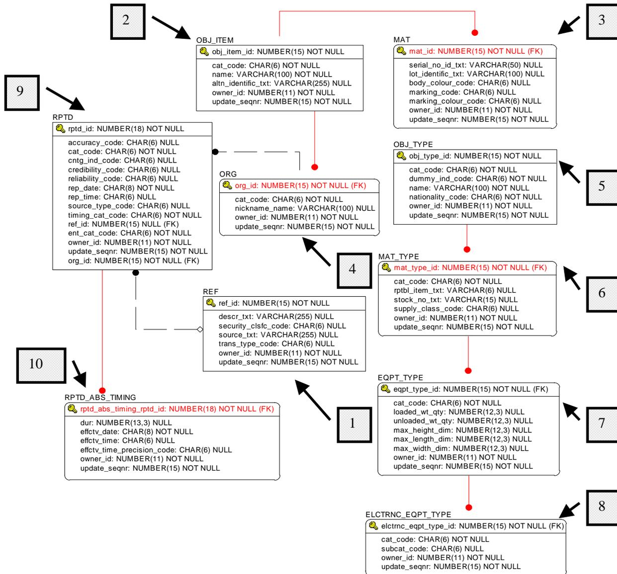
**Figure 1:** Shown here are 10 tables used in the initial filling of the LC2IEDM database with the contact data from Table 2. IDEF1X notation [6] is used to illustrate the entity-relationship diagram. The following notes apply to the numeric identifiers in the figure.
