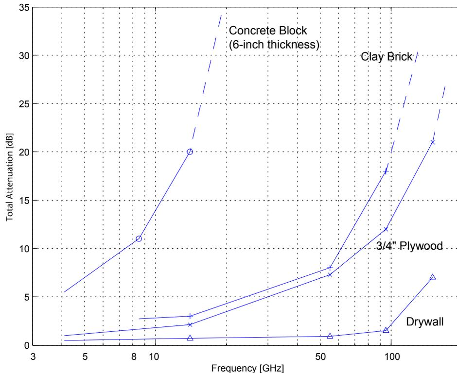
**Figure 1.** Total one-way attenuation of RF energy transmitted through various building materials. (Adapted from [6])
