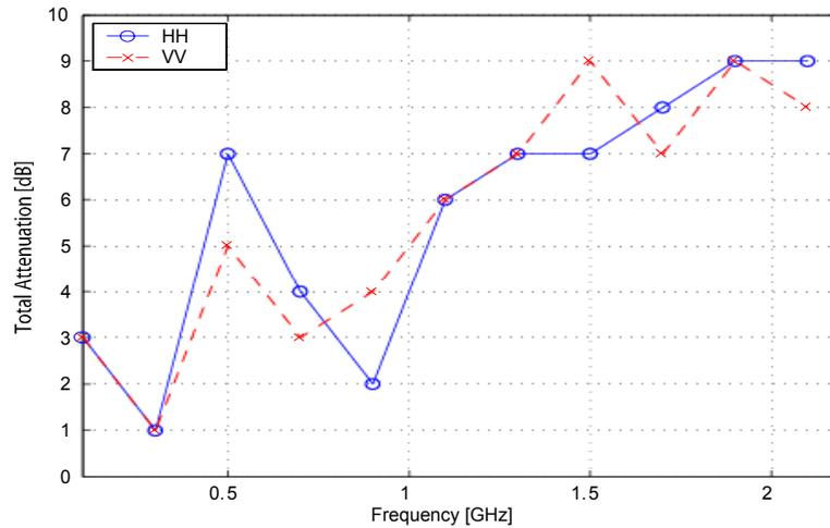
**Figure 2.** One-way loss of RF energy transmitted through 8" reinforced concrete. (Adapted from [6])
