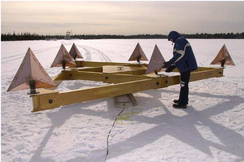
Figure 2 A photograph of the delta-wing shaped Target Motion Simulator apparatus.
