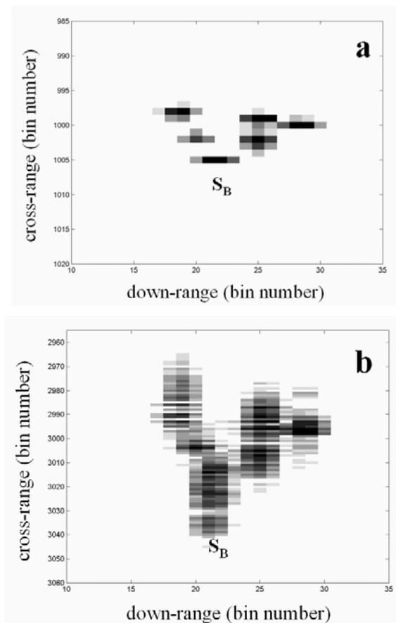
Figure 5 ISAR images of the Target Motion Simulator. a) undistorted image, b) distorted image.
