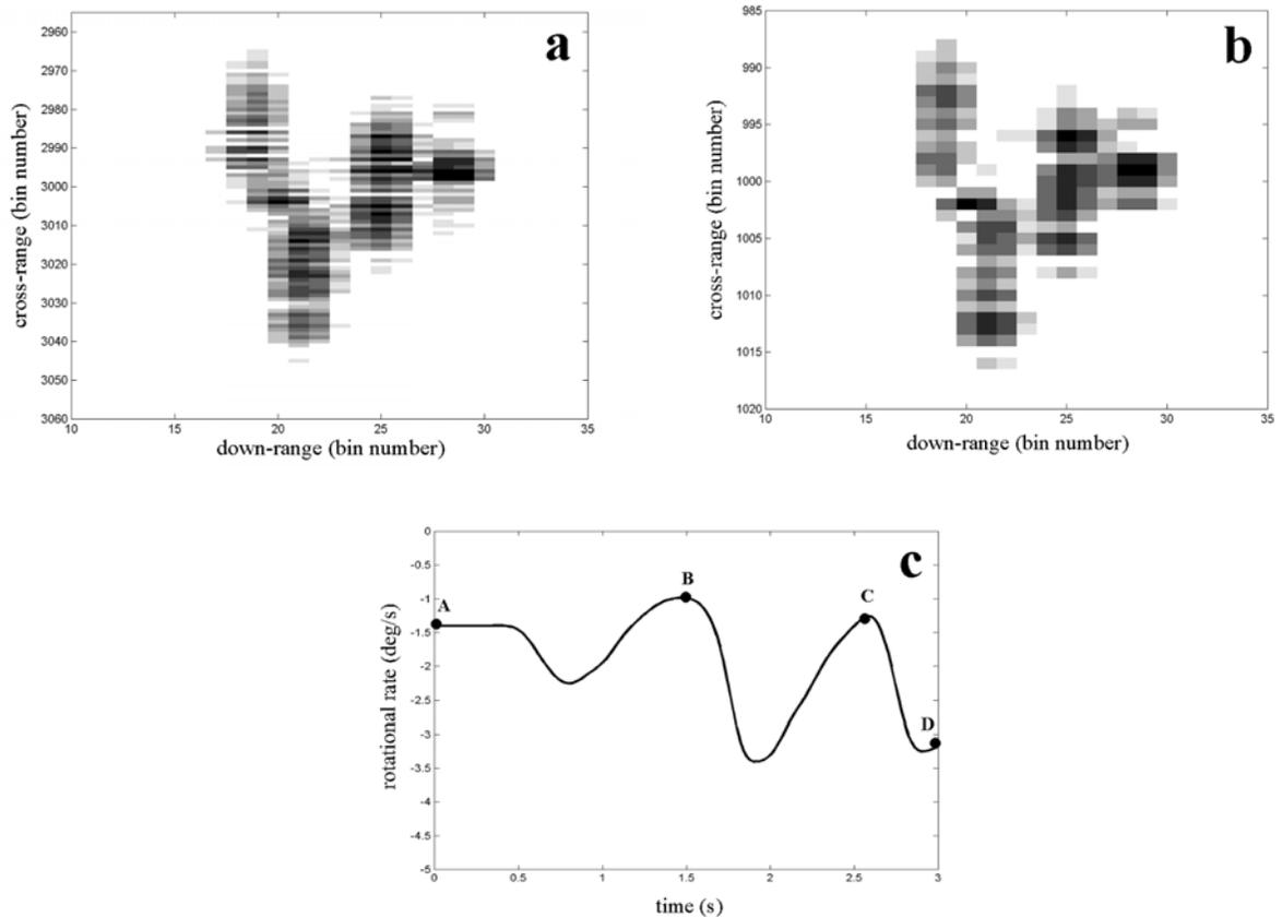
Figure 8 Distorted ISAR images processed using different image integration durations. a) image integration time = 3 seconds (A to D). b) image integration time = 1 second (B to C). c) temporal history of the TMS's motion.
