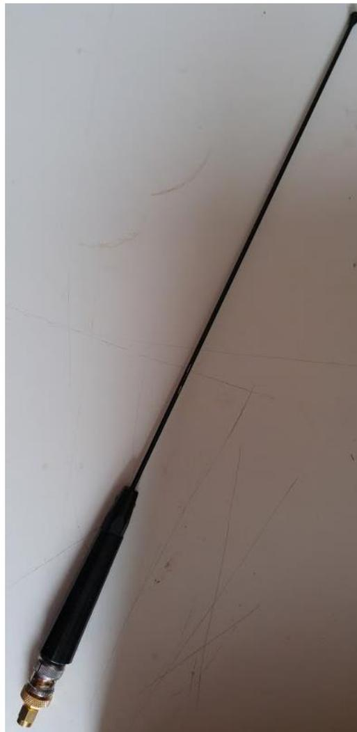
Figure 2. Monopole antenna.
