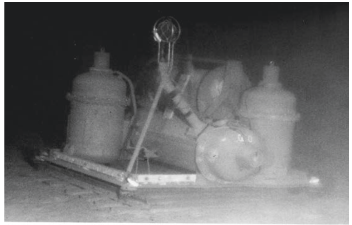
Figure 5. Photo of the Remote Instrument Package (RIP) in Lancaster Sound, Baffin Bay, Nanavut, Canada, before it was raised to the surface. The hydrophone is in the cage at the top of the package. Batteries and electronics are in the pressure vessels. The winch carrying the recovery rope is visible at the back. Photo courtesy of Canada, Department of National Defence.
