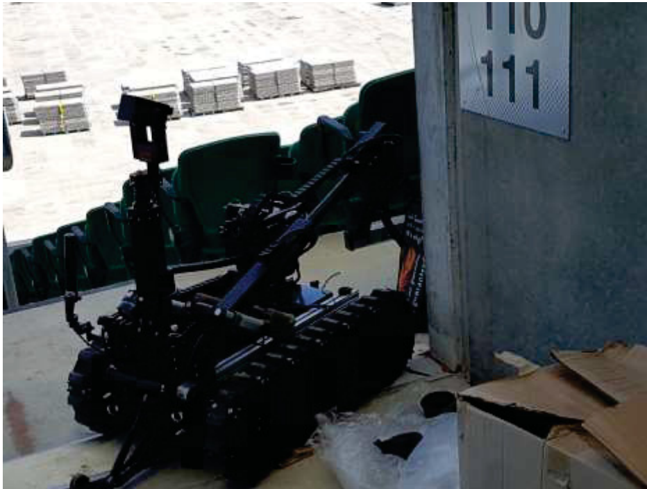
Figure 2: RPS EDU robot retrieving the suspicious package
