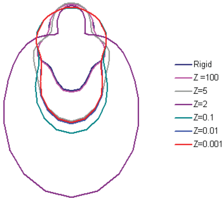
Figure 5.4. Variation of Target Strength due to Changes in Impedance: Polar Plot (480Hz)
