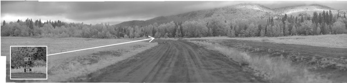
Figure 5: Final large FOV SWIR image insert showing close-up of the E-letter target.
