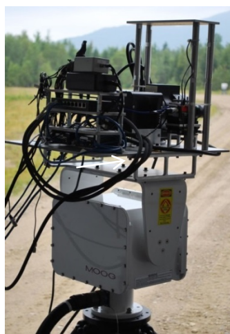
Figure 4: Close-up view of the cameras, cables and the pan-and-tilt stage.
