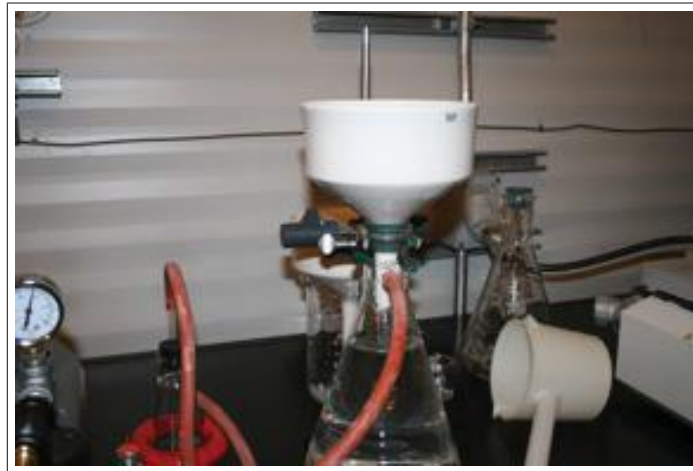
Figure 2: Paper filter arrangement for removing solid particles.
