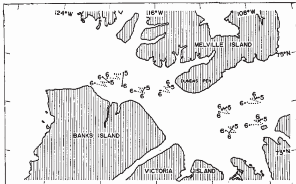
FIG. 4. Comparison of the observed buoy positions on overflight 5 (21 July) and overflight 6 (4 August) with the calculated buoy motion between these dates.
