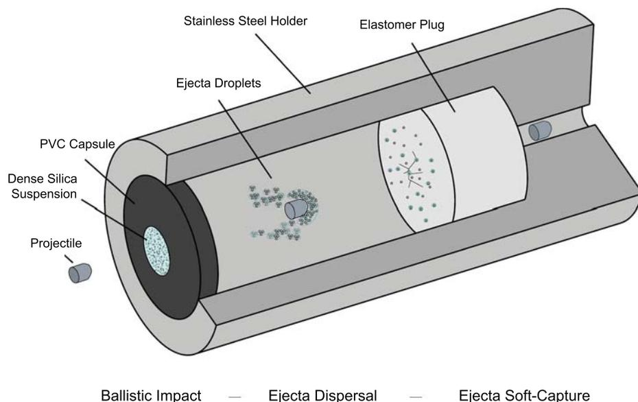
FIG. 6. A schematic of the experimental configuration sequentially prior to impact, during the projectile exit and ejecta dispersal phase, and soft-capture phase.
