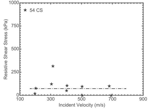
FIG. 3. The average resistive shear stress as a function of impact velocity for suspensions containing cornstarch.
