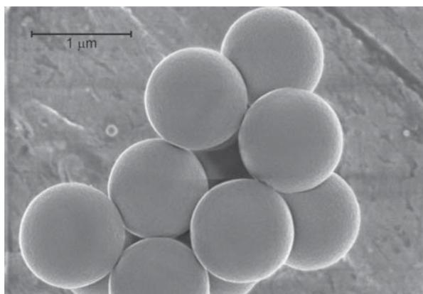
FIG. 7. SEM micrograph of the benchmark silica particles.
