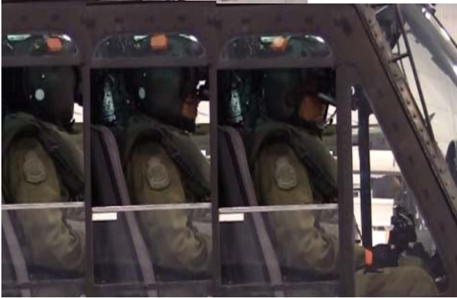
Figure 1: “Outside Scan Regular” postural sequence shows FP with NVGs at 3 time intervals. Orange device mounted on helmet is one of 17 motion capture sensors.
