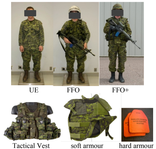
Figure 1. CIE Conditions UE, FFO and FFO+ (above). Canadian Tactical Vest, Fragmentation Protective Vest (soft armour) and ceramic plates (hard armour) (below).
