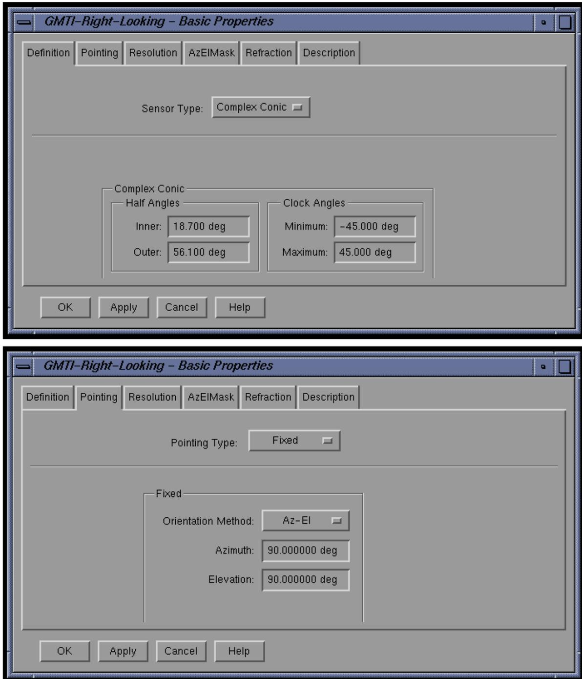
Figure 18. STK Parameters of the SMTI sensor.
