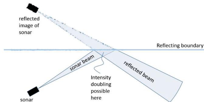
Figure 4 Schematic diagram of specular reflection of the sonar beam.
