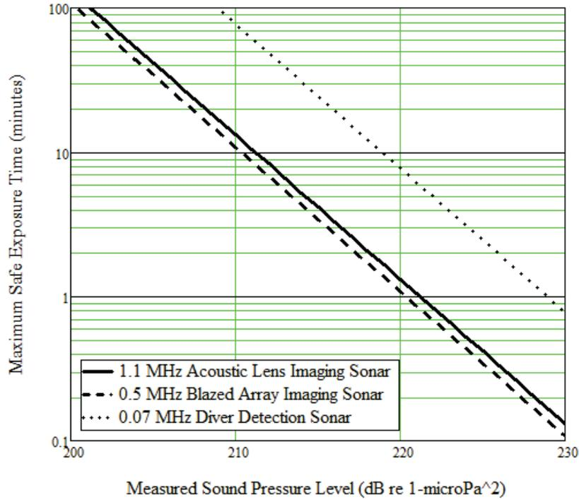
Figure 2 Maximum safe exposure time  $\Delta t$  (with no cooling mechanisms at work) as a function of the measured free-space sound pressure level  $SPL$  for the three sonars in Table (2).
