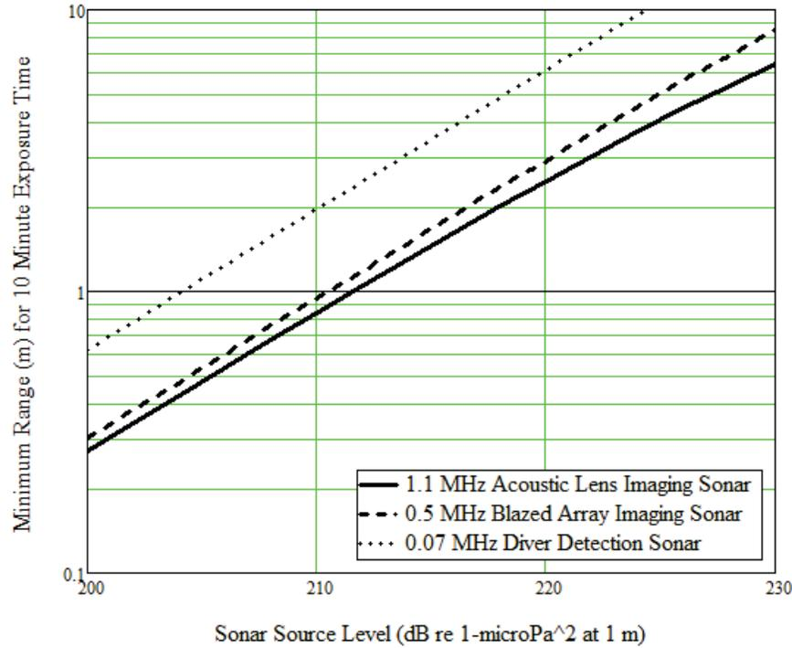
**Figure 3** Minimum safe range  $R$  on the axis of the sonar for a continuous exposure time of  $\Delta t = 10$  minutes (with no cooling mechanisms at work) as a function of the sonar source level  $SL$  when viewed in the far field from a point on the axis of the sonar beam.
