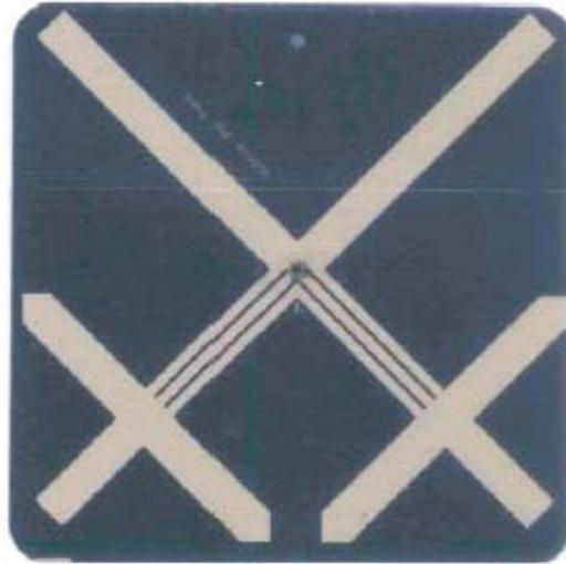
Figure 4: A dual-dipole passive RFID tag; tag size is roughly 9×9 cm.
